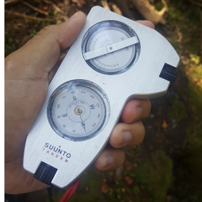
(b) Clinometer and compass for manual use.
