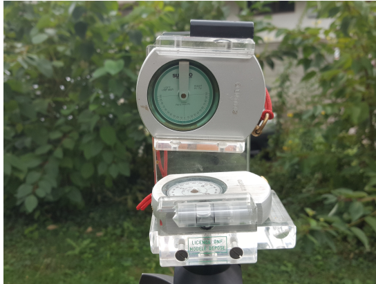
(a) Clinometer and compass for tripod
