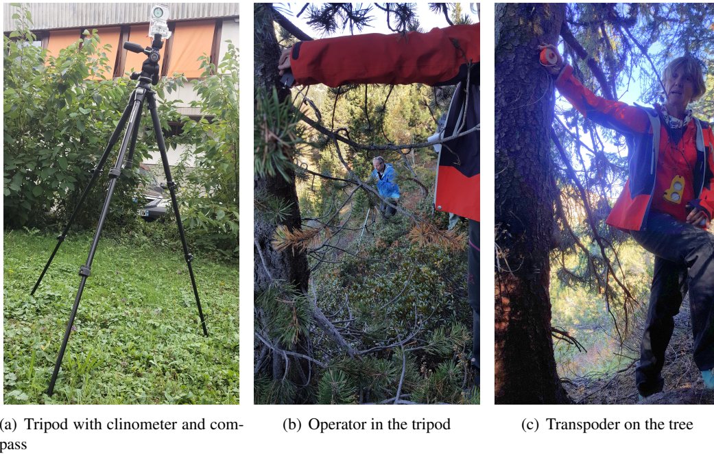
Figure 3.2: Illustration of mapping individual trees in the site of Chamrousse, France by using the tripod, clinometer, compass, hypsometer and transponder.
