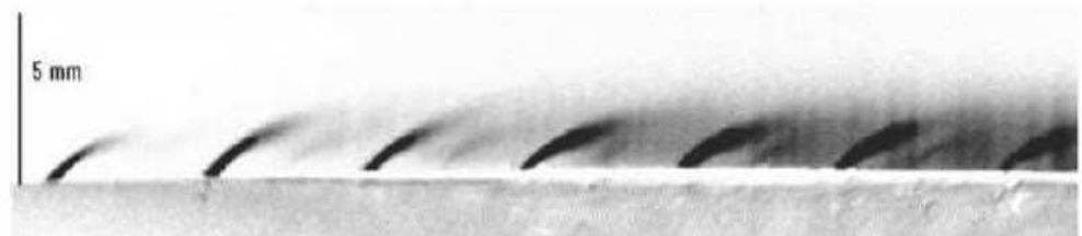
Figure 1.10: Visualisation of the film cooling using steam. Rouvreau [2001]
