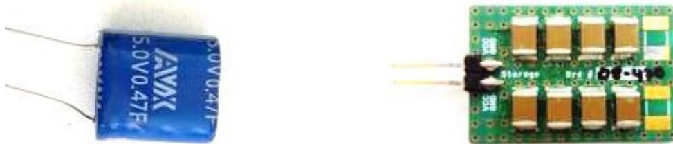
Figure 52 – Left to right: Supercapacitor and 8x ceramic capacitor array.
