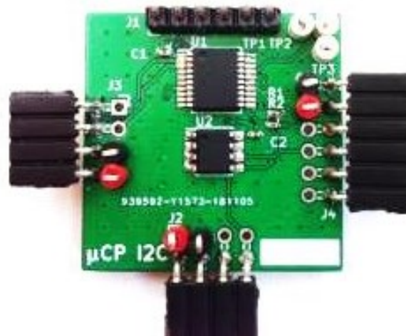
Figure 79 – Physical implementation of the microprocessor and data storage (F-RAM).
