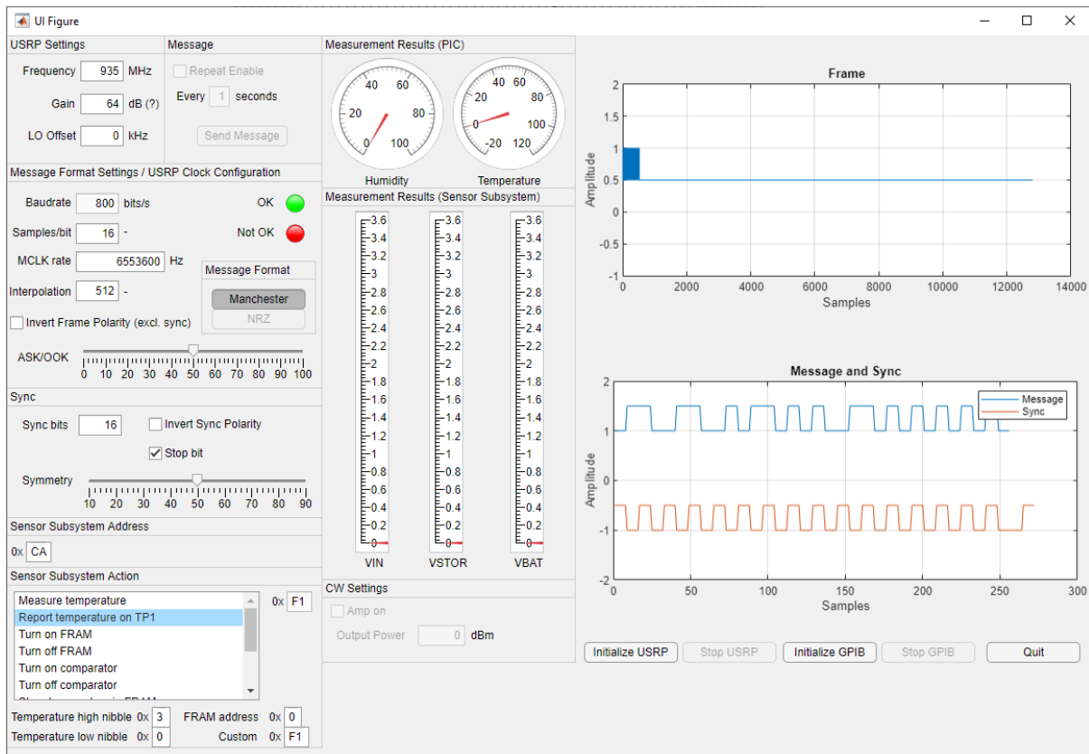
Figure 102 – GUI used in order to debug and to transmit data packets to the node.
