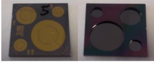
Figure 2: Optical micrograph of a chip containing different membrane sizes. Top view of the wafer (left) and back side of the wafer with cavity (right)
