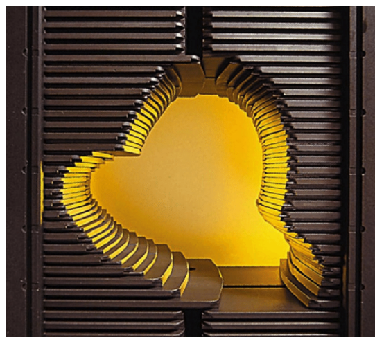
Figure 1.3: A Multi-Leaf Collimator (MLC) consists of a large number of highly absorbing tungsten leaves (on the order of 20–80 on each side) that can be positioned individually to create field openings with complex shapes. Image from Varian Medical Systems with permission.
