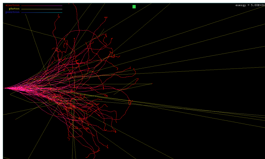
Figure 1.12: Simulation of an electron beam with initial energy of 5 MeV propagating in a water domain with a thickness of 5 cm. In red are represented the electron trajectories, in blue the positron trajectories and in yellow the photon trajectories. The simulation has been performed with the PENELOPE shower.exe program.
