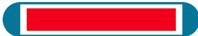
Figure 6.1: Geometry of a Nucletron SelectSeed brachytherapy source. In red the cylindrical silver rod coated with a silver halide layer (AgCl/AgI) and in blue the titanium encapsulation. Image from CLRP TG-43 Parameter Database for Brachytherapy, with permission.
