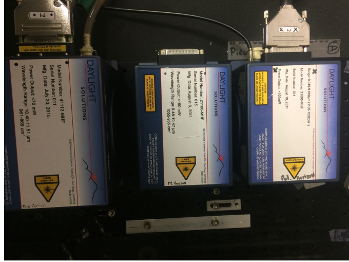
Figure 4.2.5.: A photo of mid-IR laser sources used in s-SNOM.
