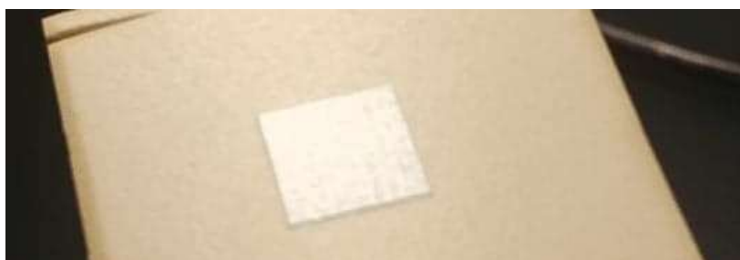
Figure 40 – Flat white sample printed with white ink used in 2.5D printing, and displaying a glossy aspect
