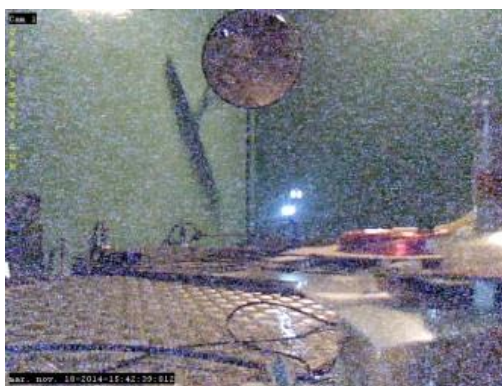
Fig. 1: Typical image degradation observed on COTS camera at low TID (<10 kGy). Figure from [9].
