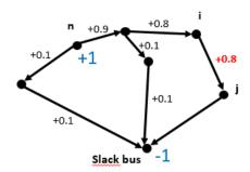
FIGURE 2.3 – Power Transfer Distribution Factors, un exemple
