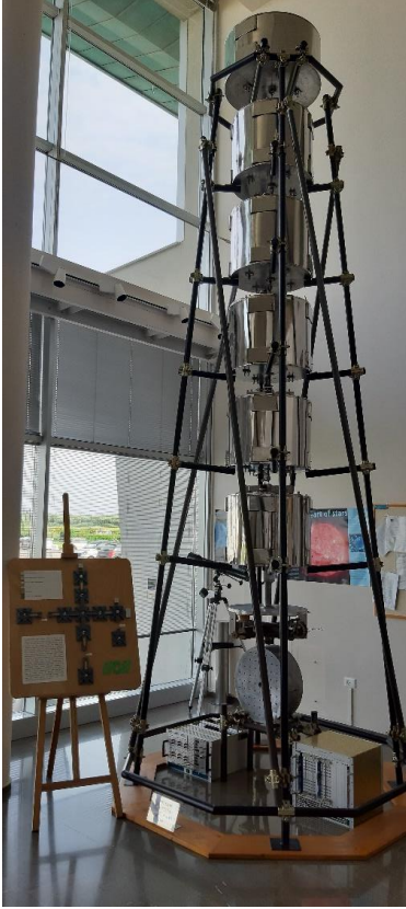
Fig. 4.6.1.l. A superattenuator on display in the Main building to show what is inside the towers. Source: Philippe Vincent
