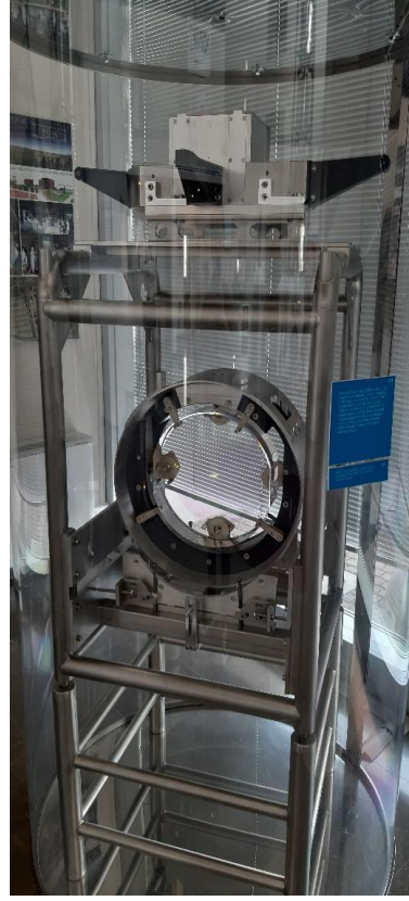
Fig. 4.6.1.m. The “marionetta” holding a mirror suspended by the monolithic silica fibers on display in the Main building. Source: Philippe Vincent
