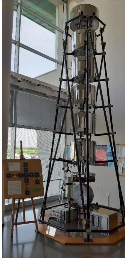
Fig. 9 A superattenuator on display in the Main building to show what is inside the towers. The superattenuators structures can be subdivided into three principal parts: the inverted pendulum (referred to as IP); the chain of seismic filters starting at filter0 to filter7 (the steering filter); and the payload (the marionette, the reference mass, and the mirror) The “marionette” is holding a mirror suspended by monolithic silica fibers.
