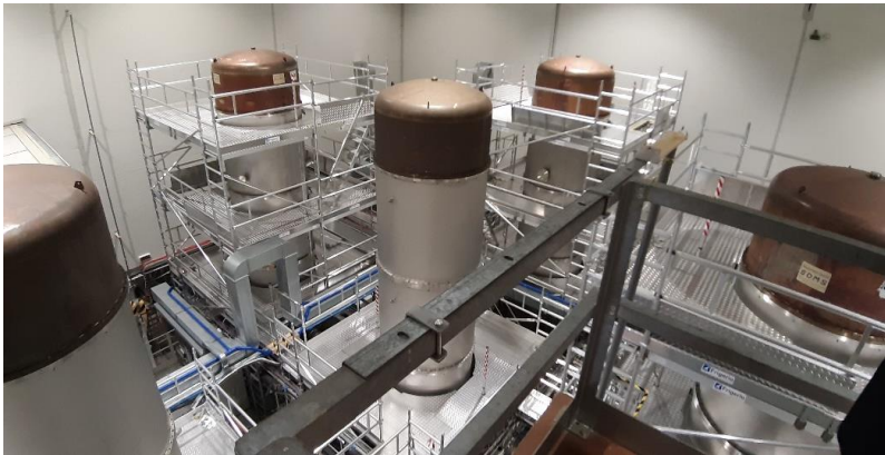
Fig. 8 Towers containing the superattenuators and the mirrors. The 5 towers are under vacuum and each contain a superattenuator from which the mirrors are suspended and controlled by the marionette. The towers from left to right contain the: Power Recycling Mirror, (West) Input Mirror, Beam Splitter, (North) Input Mirror, Signal Recycling Mirror. Source: Photo taken by Philippe Vincent
