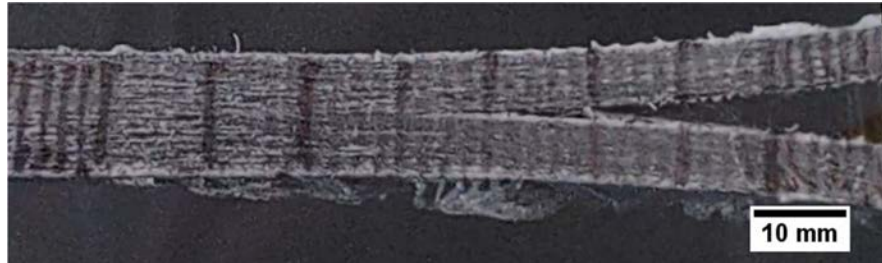
Figure 76 : Typical load-displacement curves for cCF/PA6-I with walls (a), without walls (b) and side view of cCF/PA6-I during delamination test.
