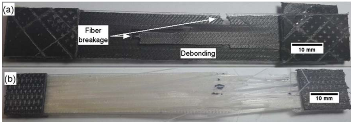
Figure 74 : Optical images of fractured (a) cCF/PA6-I and (b) cGF/PA6 showing the mode of fracture for each sample that results in fiber breakage and debonding between printed beads.
