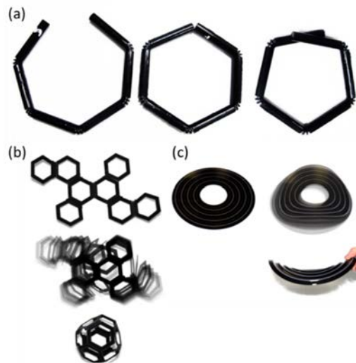
Figure 39 : 4D printing of cross-linked hygro-sensitive hydrogel and rigid plastic insensitive to water. Demonstration with self-folded lines with customized angles (a), transformation of flat surface to a 3D octahedron (b) and curved surfaces (c) [198].
