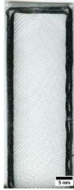
Figure 93 : Configurations of printed patterns. Two pattern families of patterns were investigated; the longitudinal pattern, with several L/W ratios, i.e 0.5 (a); 1 (b) and 2 (c); and the transverse pattern with 0.25 (d), 1 (e) and 2 (f) L/W ratios. A contouring strategy with a minimum of carbon fibers was also studied (g).
