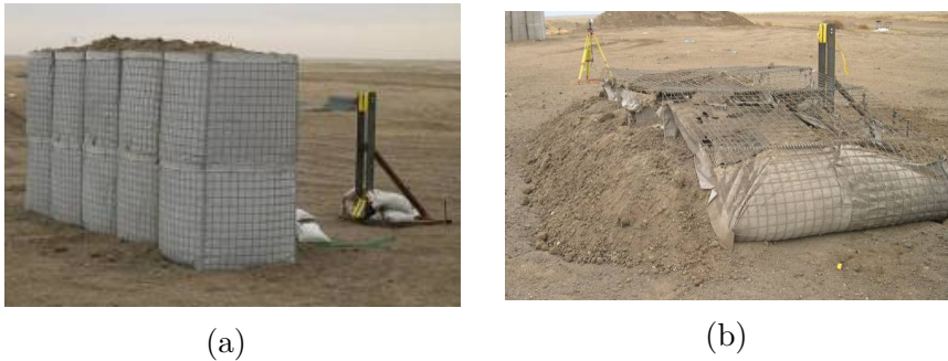
Figure 3.13 – Free-standing soil-filled containers from Scherbatiuk (2010): (a) experimental set-up and (b) overturning of the target.
