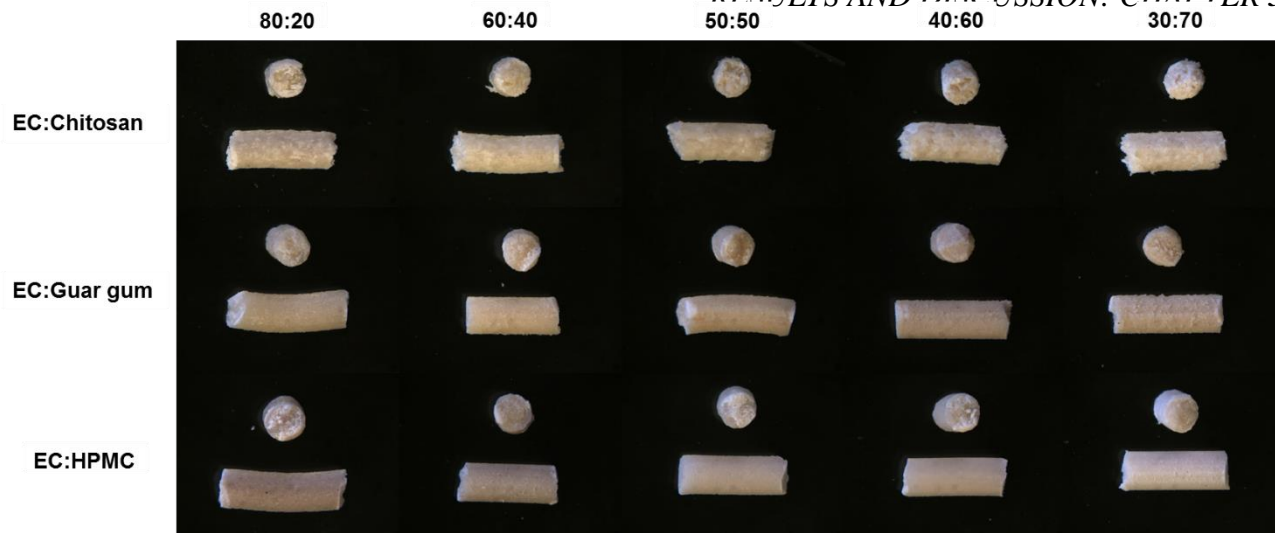
Figure 43: Macroscopic pictures of hot melt extrudates (cross-sections and surfaces) based on ethylcellulose and different types of a 2nd polymer (indicated in the figure). The polymer:polymer blend ratio was varied as indicated in the figure, the extrudates were extruded at 100 °C, loaded with 10 % theophylline and plasticized with 30 % DBS (referring to ethylcellulose).
