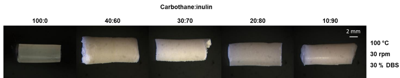
Figure 31: Macroscopic pictures of hot melt extrudates based on carbothane:inulin blends. The polymer:polymer blend ratio was varied as indicated, the extrudates were extruded at 100 °C and plasticized with 30 % DBS (referring to carbothane). For reasons of comparison, also hot melt extrudates based “only” on carbothane (plasticized with 30 % DBS) are illustrated.
