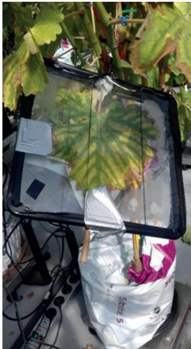
**Fig. B1.1.** Experimental set-up for ethylene sampling during esca leaf symptom expression.
