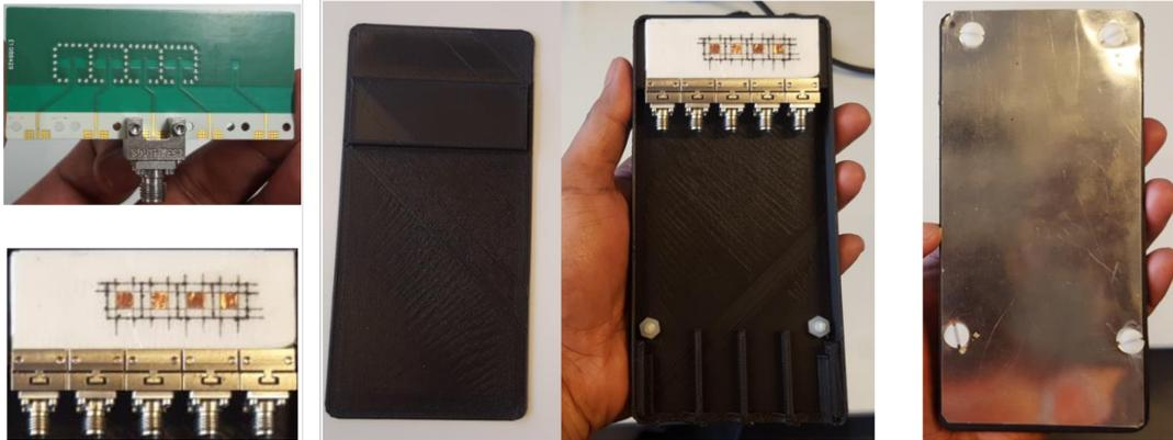
FIGURE 5.12: The simplified mobile phone prototype with antenna array and casing.
