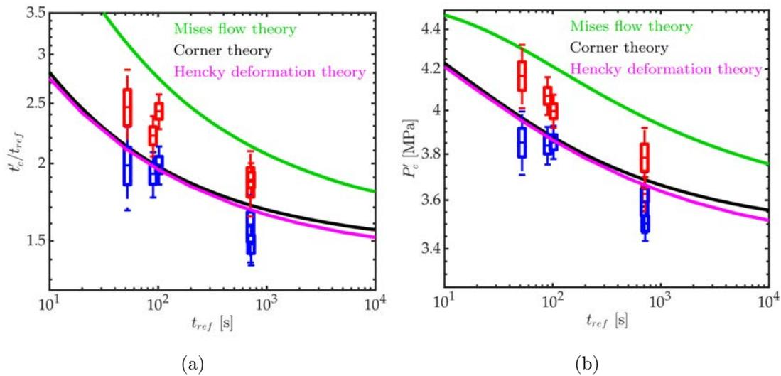
**Figure 5.35:** (a) Comparison of the three prediction methods with the projected experimental critical time ratio; (b) Comparison of the three prediction methods with the projected experimental critical pressures.
