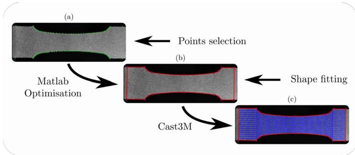
**Figure D.2:** DIC mesh fitting for FEMU method
