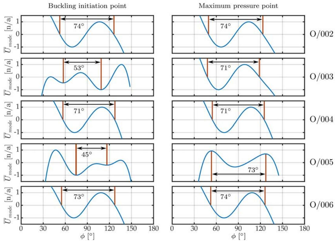
**Figure 5.23:** Normalized buckling modes on the section of biggest radius for all specimens at the buckling initiation point and at the maximum pressure point
