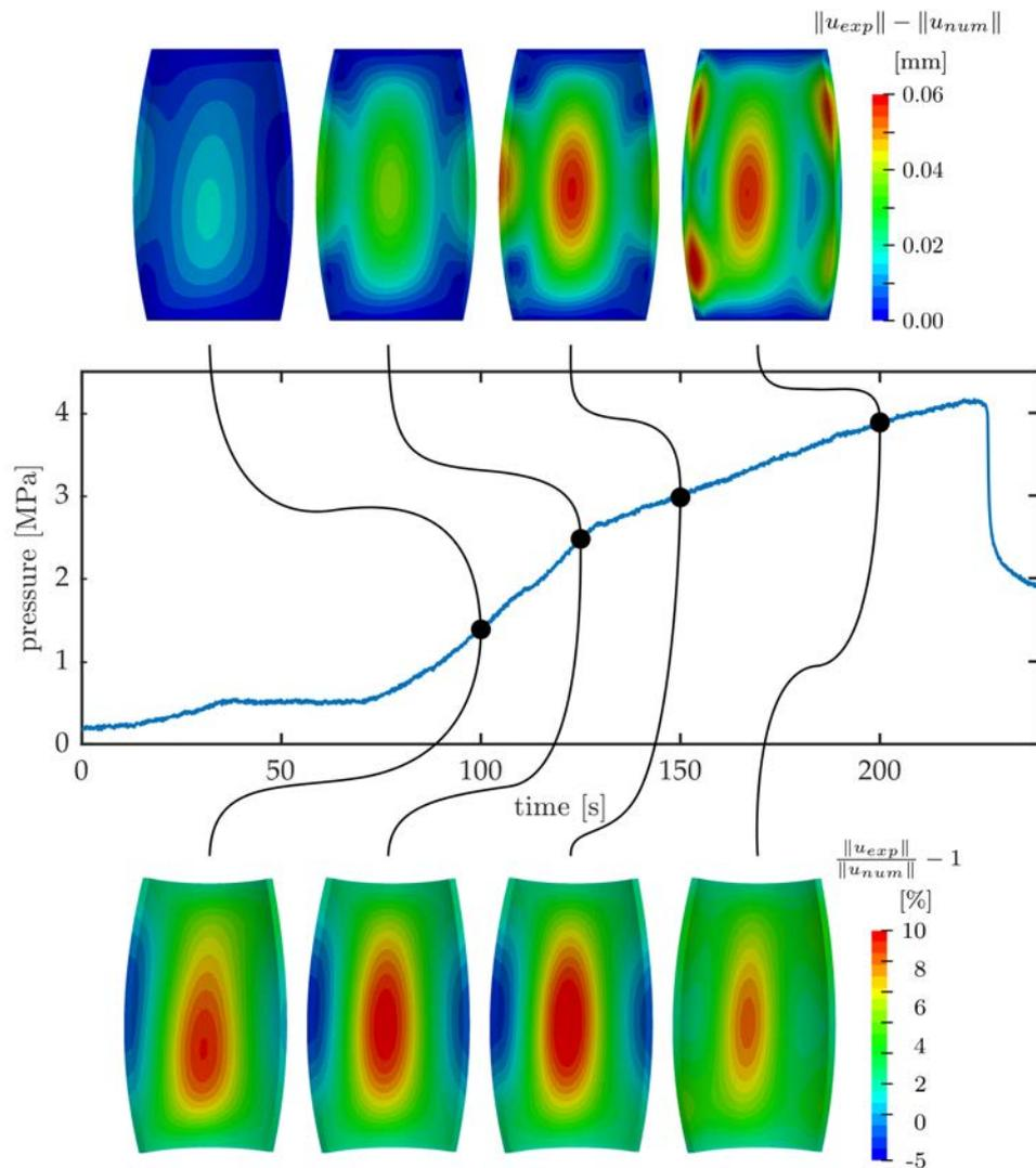
**Figure 5.24:** Absolute and relative errors between numerical and experimental displacements after the identification of  $\Delta R_0$  (O/003).
