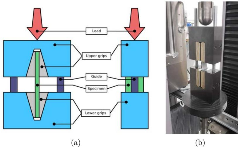
**Figure 2.12:** (a) Experimental set-up for plate buckling; (b) Experimental set-up in the testing machine, with a buckled specimen
