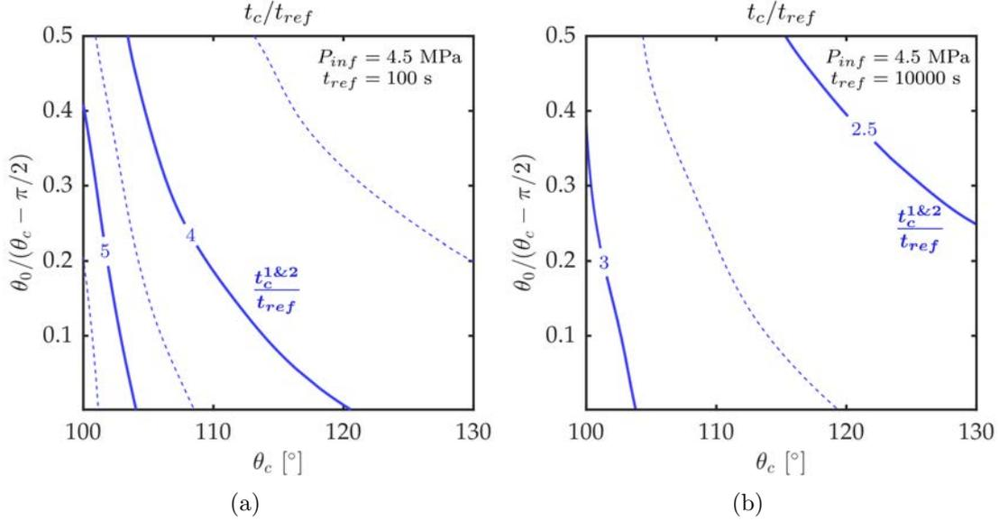
**Figure 5.9:** (a) Evolution of the first ( $t_c^{1\&2}$  blue iso-values) critical time ratio with respect to  $\theta_c$  and  $\theta_0$  for a pressure profile defined by  $P_{inf} = 4.5$  MPa and  $t_{ref} = 100$  s; (b) Evolution of the first ( $t_c^{1\&2}$  blue iso-values) critical time ratio with respect to  $\theta_c$  and  $\theta_0$  for a pressure profile defined by  $P_{inf} = 4.5$  MPa and  $t_{ref} = 10000$  s
