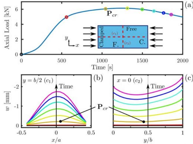
**Figure 4.2:** Evolution in time of the experimental out of plane displacement field on both center lines  $x = 0$  and  $y = b/2$  of the plate (Specimen BT1/01: plate dimensions  $a = b = 40\text{mm}$  and  $h = 4\text{mm}$ )
