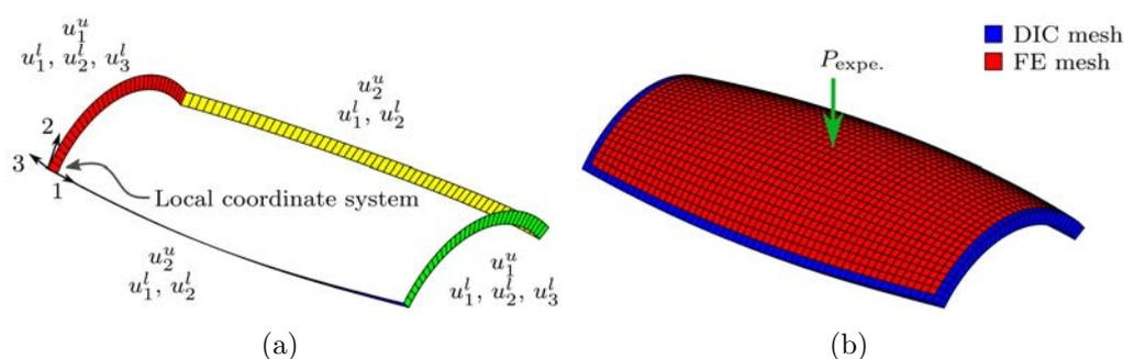
**Figure 2.22:** (a) Enforcement of experimental boundary conditions on the FE mesh, subscript  $^l$  for lower skin and  $^u$  for upper skin; (b) the FE mesh is equal to the DIC mesh with a mesh row removed on each edge, experimental pressure is applied on the FE mesh.
