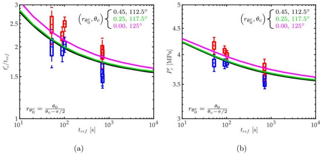
**Figure 5.34:** (a) Comparison of the projected experimental critical time ratio with the numerical predictions for three values of  $\theta_0$ ; (b) Comparison of the projected experimental critical pressures with the numerical predictions for three values of  $\theta_0$ .
