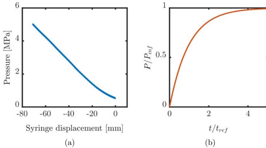
**Figure 2.20:** (a) Relation between the syringe displacement and the tank pressure; (b) Parametric pressure history applied to egg shell
