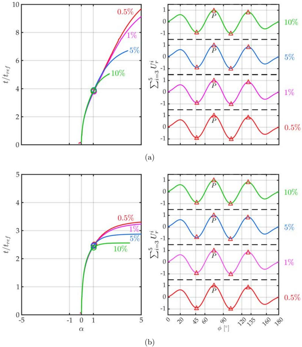
**Figure 5.7:** (a) Evolution of the singular solution  $\alpha$  with respect to time and the imperfection amplitudes (left); approximation of the singular solution for each imperfection amplitude (right) for  $t_{ref} = 100$  s; (b) Evolution of the singular solution  $\alpha$  with respect to time and the imperfection amplitudes (left) approximation of the singular solution for each imperfection amplitude (right) for  $t_{ref} = 10000$  s
