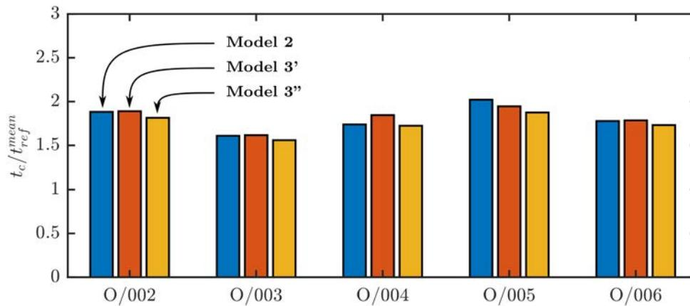
**Figure 5.29:** Effect of the imperfections on the boundary conditions on the predicted critical time ratio for all specimens; for **Model 3'**  $A_p = 0.275 \text{ mm.MPa}^{-1}$ ; for **Model 3''**  $K = 2000 \text{ N.mm}^{-1}$
