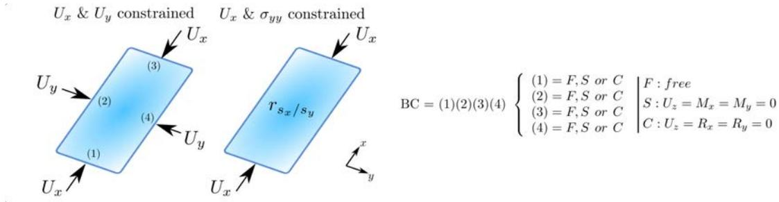
**Figure 2.10:** Definition of the plate buckling problem;  $F$ ,  $S$  and  $C$  for free, simply supported and clamped;  $M_x$  and  $M_y$  the moments around  $x$  and  $y$  axis respectively;  $R_x$  and  $R_y$  the loads along  $x$  and  $y$  axis respectively
