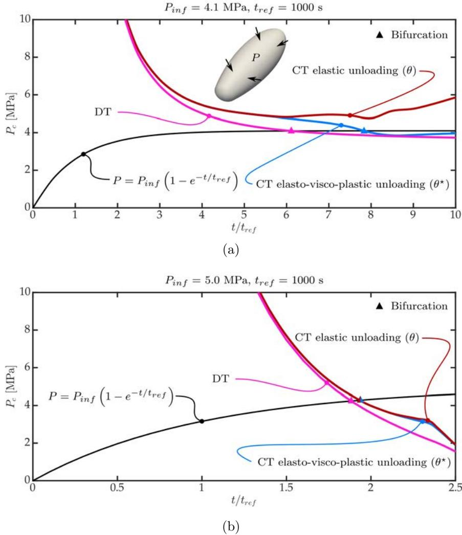
**Figure 2.9:** (a) Comparison of the eigen pressure from corner theory (CT) for both unloading criteria with the eigen pressure from the deformation theory (DT) in the creep regime, (b) Comparison of the eigen pressure from corner theory (CT) for both unloading criteria with the eigen pressure from the deformation theory (DT) in the elasto-visco-plastic regime. Results from a FE simulation with the material parameters from 3.5, and  $\theta_0 = 10^\circ$  and  $\theta_c = 110^\circ$ .
