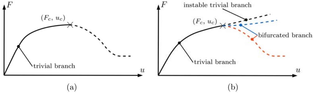
**Figure 1.7:** (a) limit point buckling; (b) bifurcation buckling
