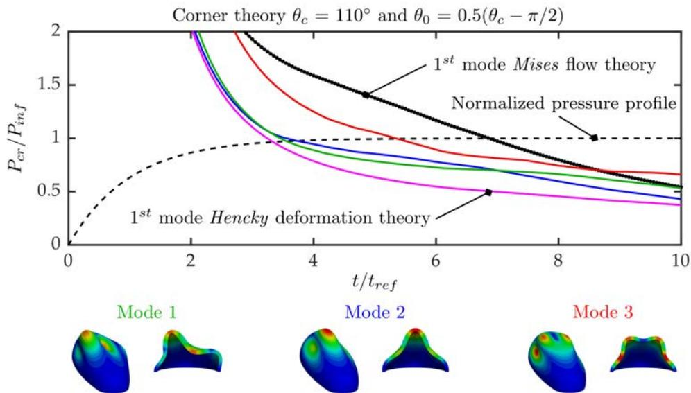
**Figure 5.8:** Evolution of the eigen pressure according to the normalized time and the three first buckling mode predicted with the corner theory for a pressure profile defined by  $P_{inf} = 4.5$  MPa and  $t_{ref} = 100$  s
