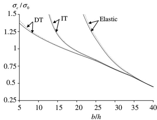
**Figure 1.11:** Normalized buckling stress versus  $b/h$  ratio for a fully clamped square plate subjected to an in-plane equi-biaxial loading (dashed curves thin plate theory, plain curves Reissner-Midlin plate theory). [Wang and Aung 2007]
