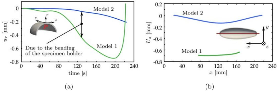
**Figure 5.26:** (a) Effect of the loading imperfection on the radial deflection  $u_r$  of a point (P) on the top on the egg (O/003), green **Model 1**, blue **Model 2**; (b) Effect of the loading imperfection on the vertical deflection  $U_z$  of an axial section of the lower skin (red line) of egg O/003), green **Model 1**, blue **Model 2**
