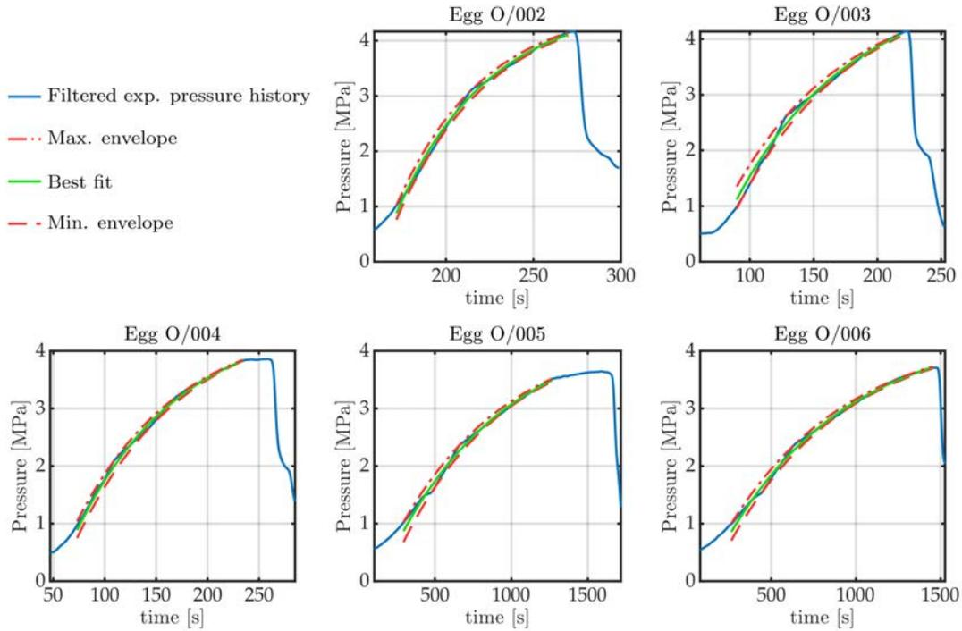
**Figure 5.13:** Pressure profiles identified for each specimen
