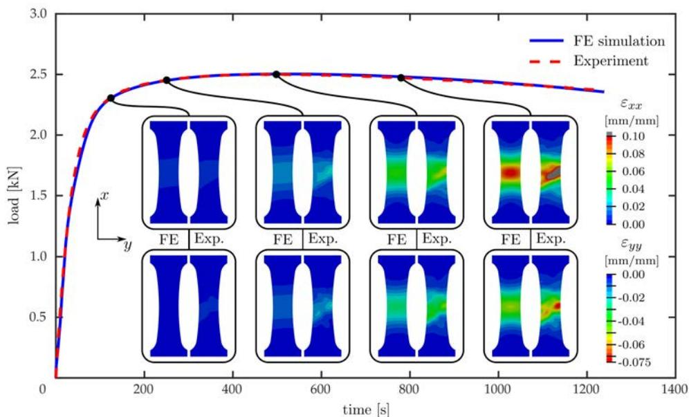
**Figure 3.7:** FE simulation vs. experiment TT/31
