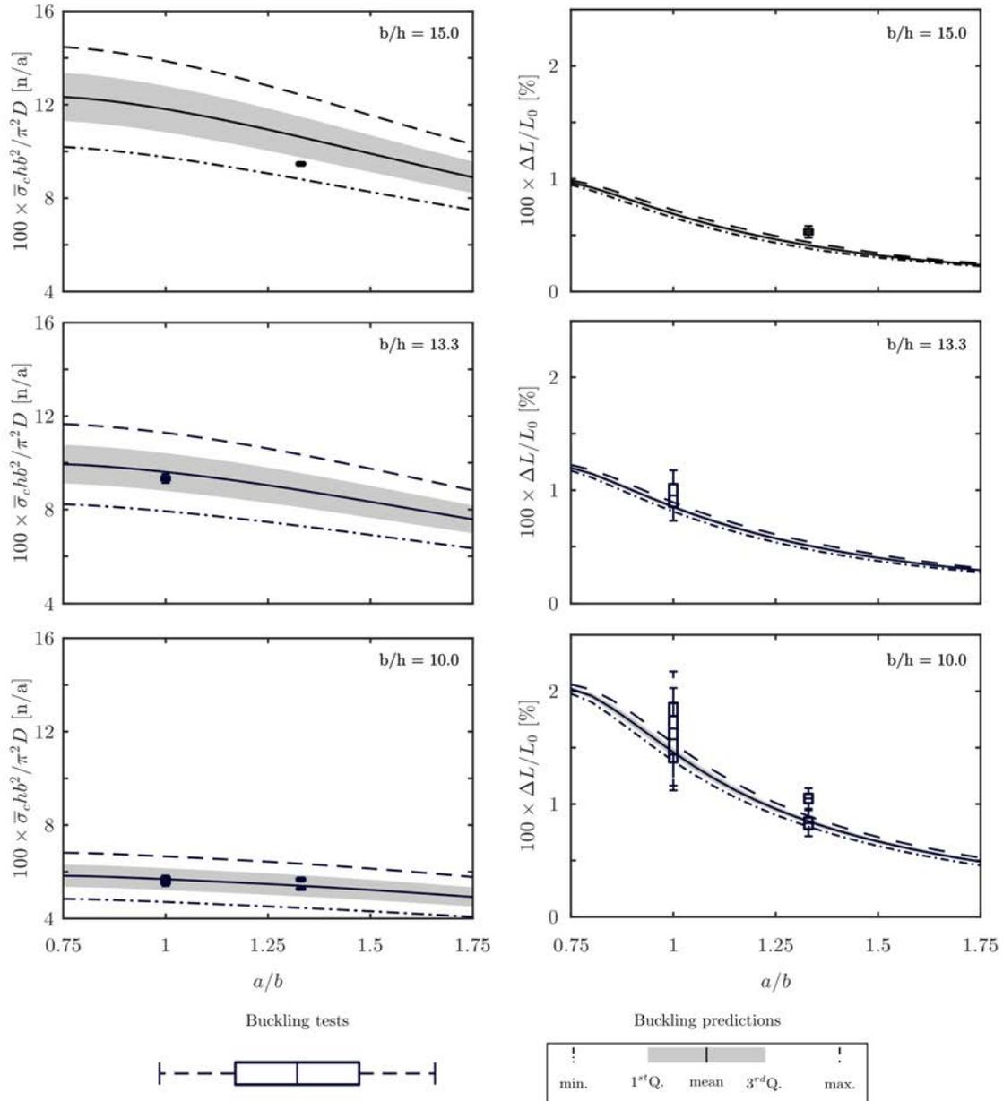
**Figure 4.9:** Analytical buckling predictions vs. experimental effective normalized critical stress (left) and critical strain (right), plotted according to the plate aspect ratio and for each plate thickness ratio
