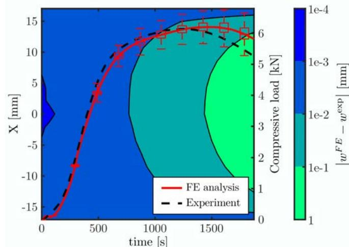
**Figure 4.7:** FEA vs. experiment for BT1/01 specimen, Evolution of compressive load and chronograph of the out of plane displacement deviation on the middle line ( $y = b/2$ ) according to time and axial coordinate  $x$
