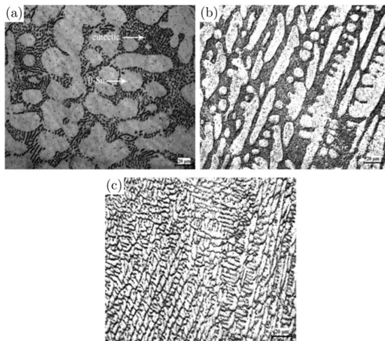
**Figure 1.2:** Effect of the cooling rate on the SAC 305 microstructure; cooling rate: (a)  $0.14^{\circ}\text{C}\cdot\text{s}^{-1}$ , (b)  $1.7^{\circ}\text{C}\cdot\text{s}^{-1}$ , (c)  $100^{\circ}\text{C}\cdot\text{s}^{-1}$  [Wei and Wang 2012]
