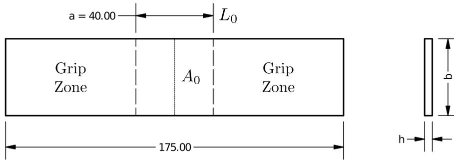
**Figure 2.11:** Plate buckling specimen drawings, dimension in mm
