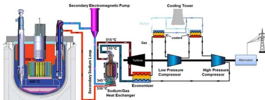
**Figure 7:** Sodium fast reactor diagram of general principle
