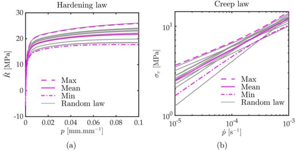
**Figure 3.10:** (a) Envelope at 95% probability with 90% of confidence of the hardening variable and random hardening laws, (b) Envelope at 95% probability with 90% of confidence of the creep equivalent stress and random creep laws
