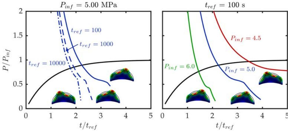
**Figure F.1:** (left) Eigen pressure ratio with respect to time ratio  $t/t_{ref}$  for different pressure rates; (right) Eigen pressure ratio with respect to time ratio  $t/t_{ref}$  for different saturating pressures ( $P_{inf}$  in MPa)
