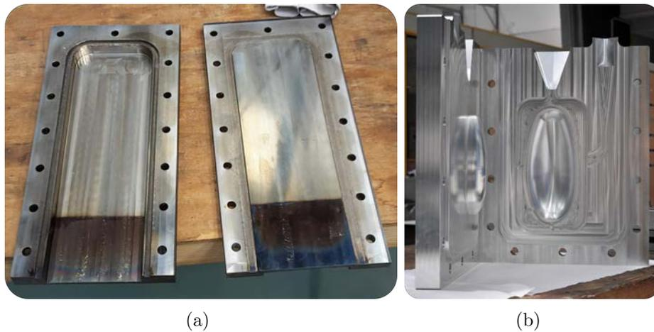
**Figure 2.3:** (a) Steel mould used to cast tensile and compressive specimens; (b) Aluminium mould used to cast externally pressured specimens
