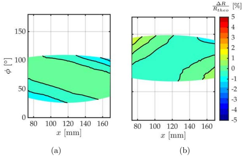
**Figure 5.17:** (a) Relative error map on the area analysed with the images of camera 0 and 1; (b) Relative error map on the area analysed with the images of camera 0 and 2 (Egg O/003)
