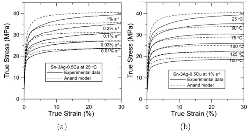
**Figure 1.4:** (a) Effect of the strain rate on the SAC 305 strength [Bai, Chen, and Gao 2009]; (b) Effect of the alloy temperature on the SAC 305 strength [Bai, Chen, and Gao 2009]
