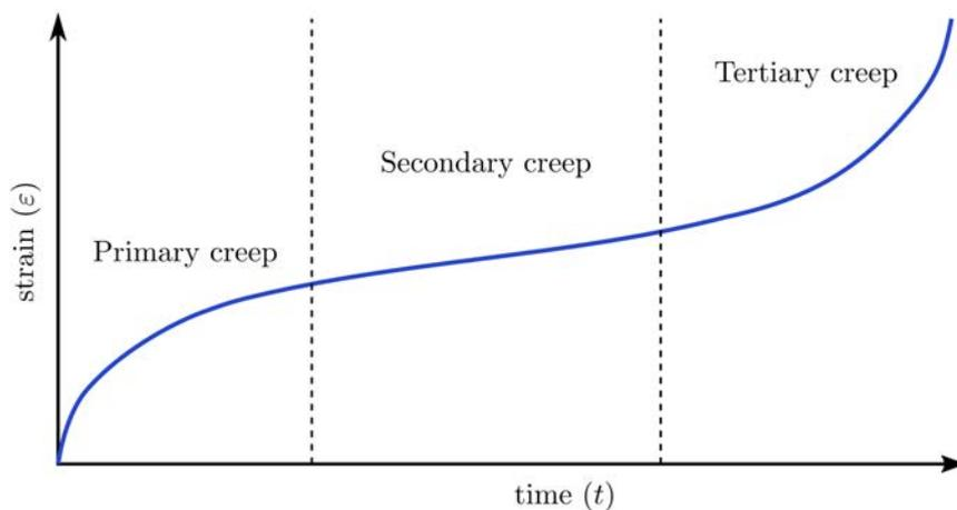
**Figure 1.5:** Identification of the three creep phases on a creep test
