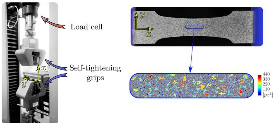
**Figure 2.6:** Tensile experimental set-up and speckle pattern
