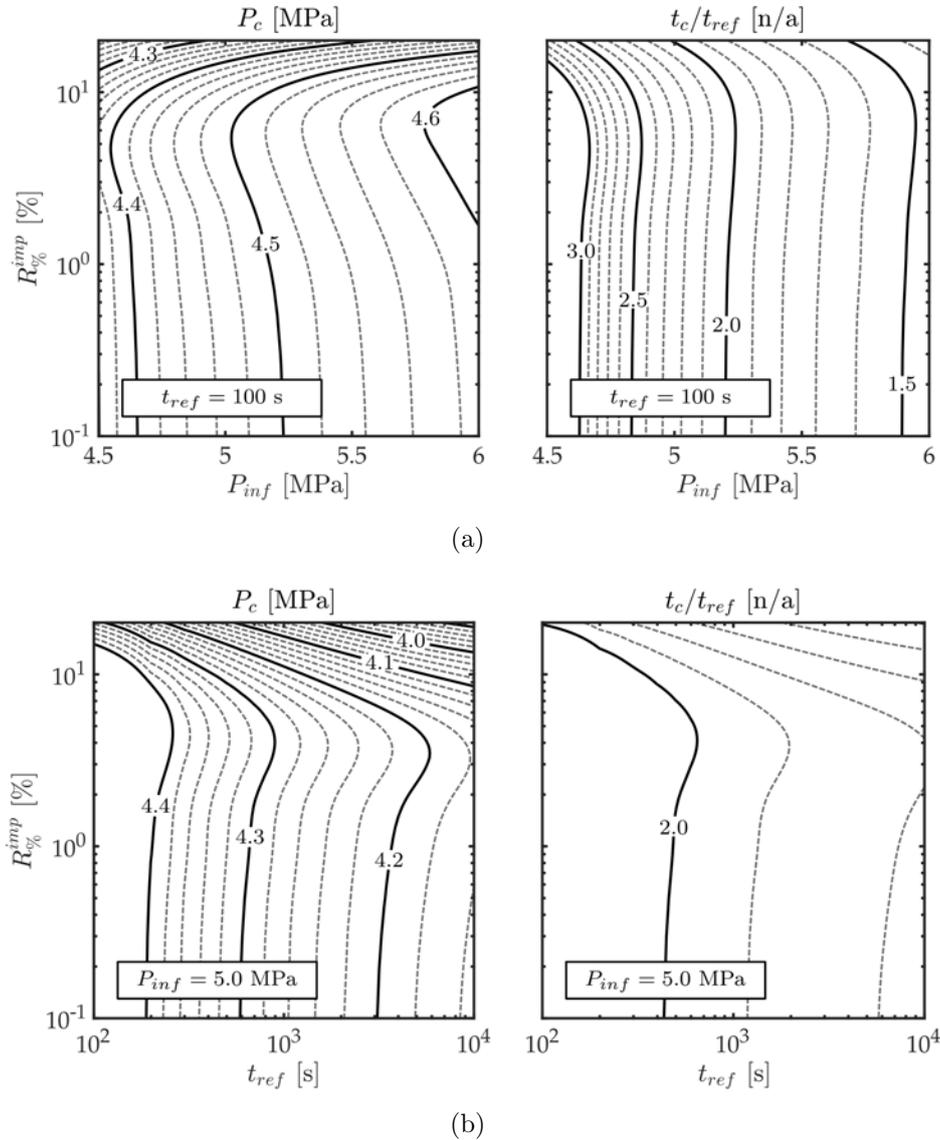
**Figure F.3:** (a) Critical pressure (left) and time ratio (right) iso-values with respect to  $P_{inf}$  and  $R_{\%}^{imp}$  with  $t_{ref} = 100$  s; (b) Critical pressure (left) and time ratio (right) iso-values with respect to  $t_{ref}$  and  $R_{\%}^{imp}$  with  $P_{inf} = 5$  MPa
