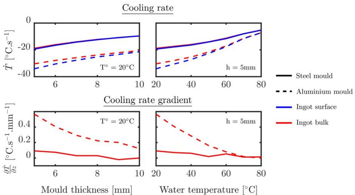
**Figure B.2:** Results of the quench parametric study; top graphs correspond to cooling rate at the surface of the ingot (in blue) and in the bulk (in red) with respect of the mould thickness and water temperature; bottom graphs correspond to the cooling rate gradient between the surface and the bulk of the ingot. Results are presented for Aluminium mould (dashed line) and steel mould (plain line)
