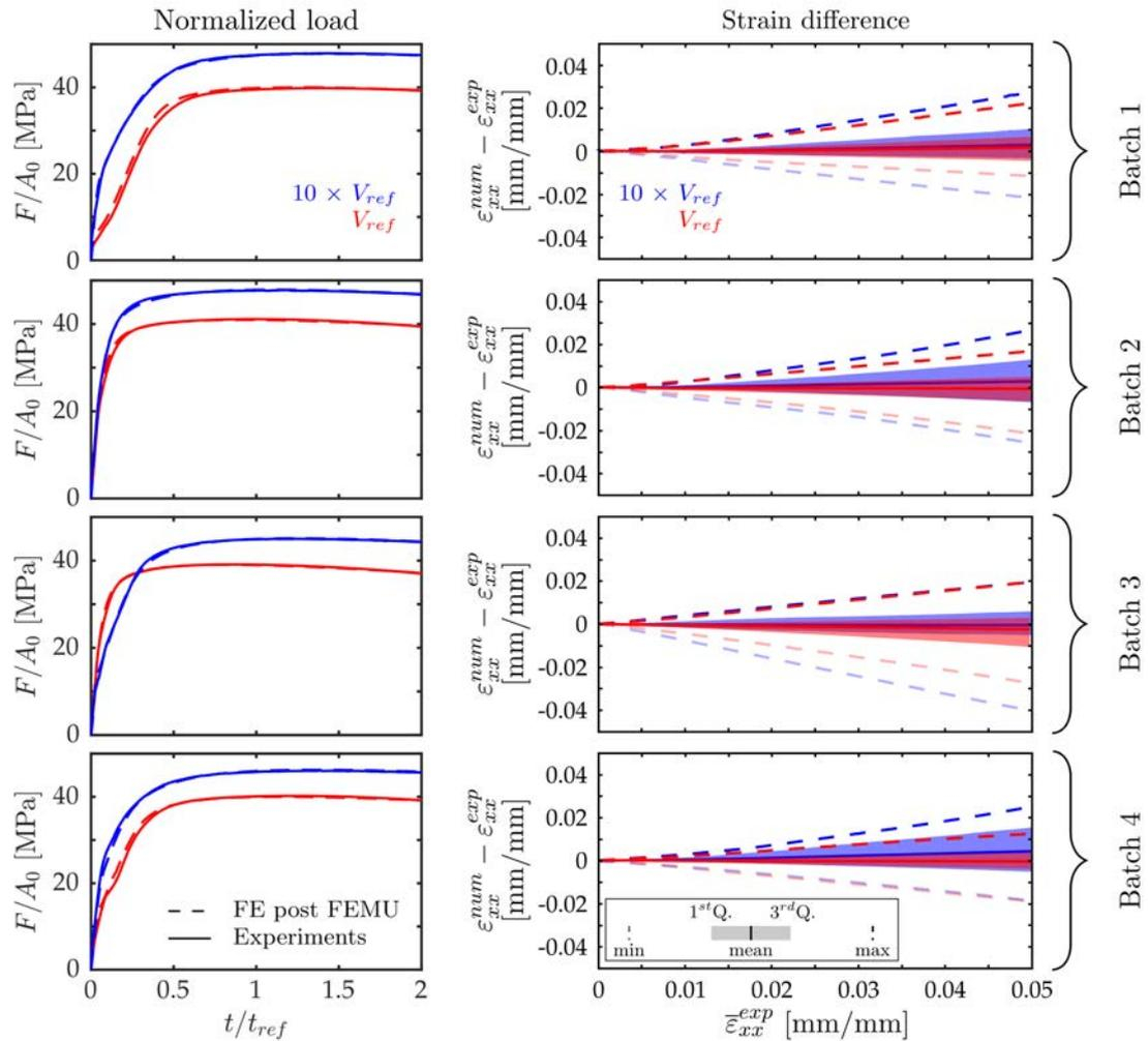
**Figure E.5:** FE post FEMU vs. experiments for all tensile experiments, (left) Normalized load with respect to the normalized time, (right) statistical description of the strain difference between FE post FEMU and experimental strain  $\varepsilon_{xx}$  with respect to the mean experimental axial strain  $\bar{\varepsilon}_{xx}^{exp}$ .
