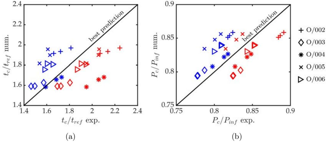
**Figure 5.31:** (a) Comparison of the experimental normalized critical times with the predicted ones; (b) Comparison of the experimental normalized critical pressures with the predicted ones; both experimental detection methods are evaluated (buckling initiation points in blue and maximum pressure point in red).
