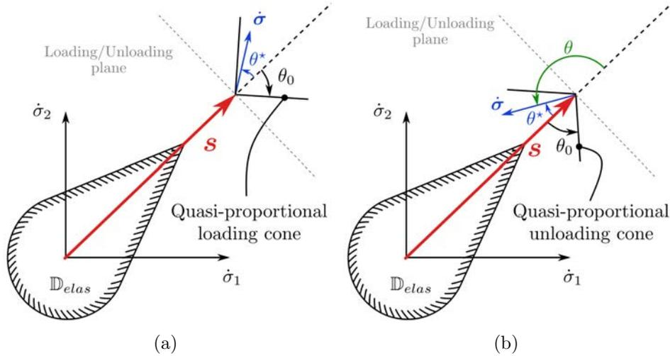
**Figure 2.8:** (a) Visco-plastic loading mechanism using the corner theory yield surface; (b) Visco-plastic unloading mechanism using the corner theory yield surface
