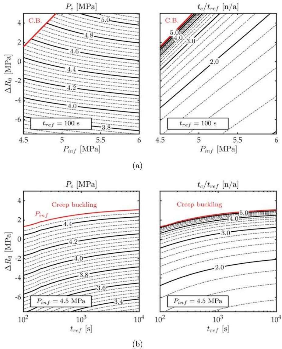
**Figure F.4:** (a) Critical pressure (left) and time ratio (right) iso-values with respect to  $P_{inf}$  and  $\Delta R_0$  with  $t_{ref} = 100$  s; (b) Critical pressure (left) and time ratio (right) iso-values with respect to  $t_{ref}$  and  $\Delta R_0$  with  $P_{inf} = 4.5$  MPa
