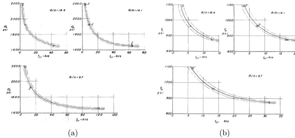
**Figure 1.14:** (a) Experimental critical compressive stress data with respect to the critical time (white bullet); (b) Experimental critical torsional shear stress data with respect to the critical time (white bullet) [Gerard and Gilbert 1958]
