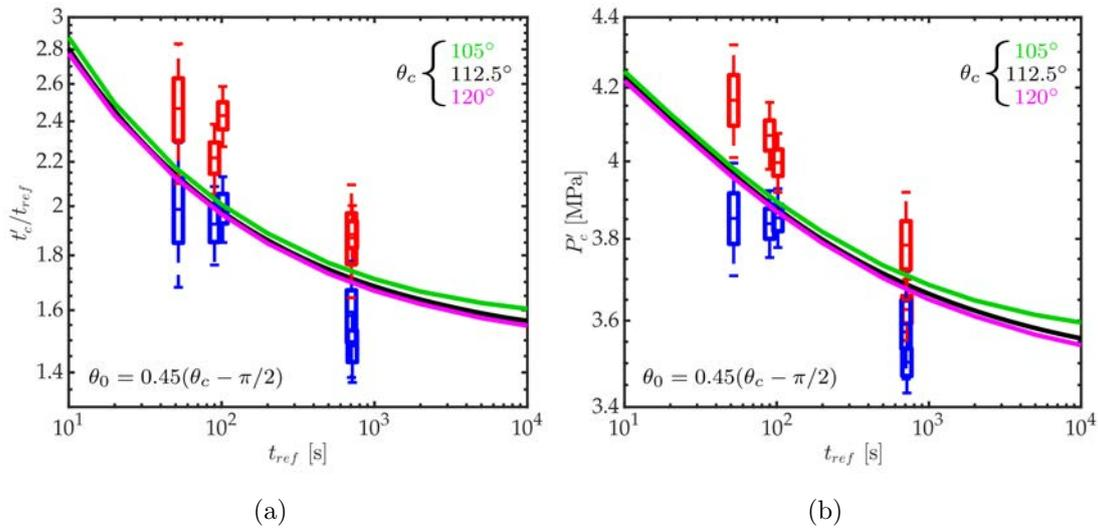
**Figure 5.33:** (a) Comparison of the projected experimental critical time ratio with the numerical predictions for three values of  $\theta_c$ ; (b) Comparison of the projected experimental critical pressures with the numerical predictions for three values of  $\theta_c$ .
