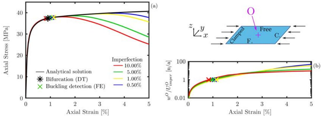
**Figure 4.6:** Buckling analysis of a square plate for various loading imperfection amplitudes, comparison of post buckling solutions (FE) and the perfect solution (analytical model); detection of buckling initiation depicted by crosses. (a) axial stress vs. axial strain, (b) imperfection ratio vs. axial strain.
