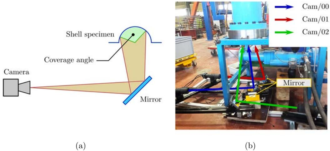
**Figure 2.19:** (a) Concept of indirect image acquisition; (b) Integration of the optical set-up in the test rig environment
