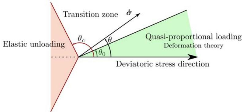
**Figure 1.12:** Description of the three loading zones around the corner of the yield surface (black curves are associated to the corner theory with two different sets of parameters  $\theta_0$  and  $\theta_c$ ).
