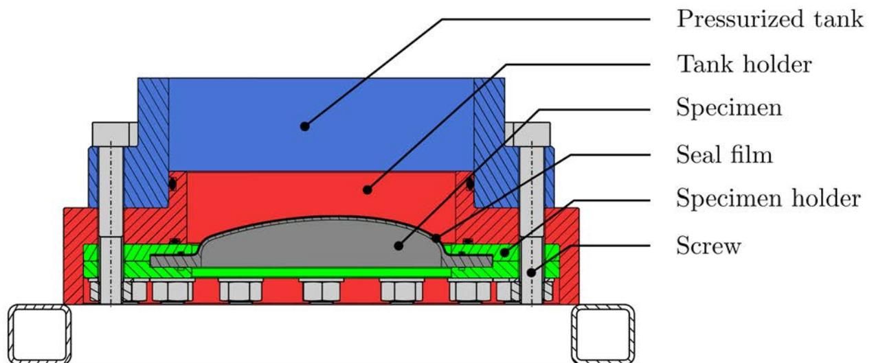
Figure 2.18: Test rig assembly with the specimen
