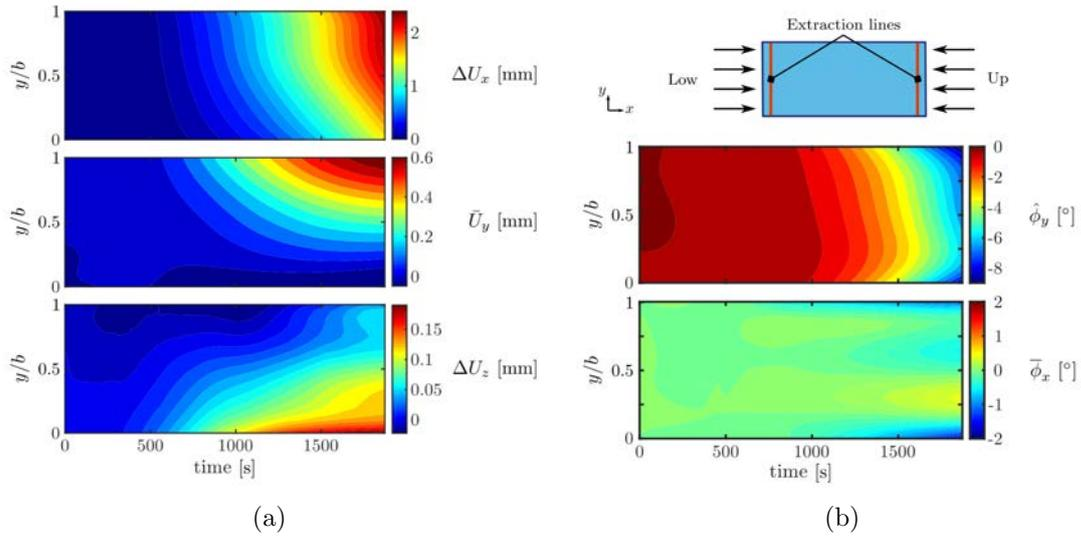
**Figure 4.4:** (a) Displacement fields characterizing the loading conditions of plate BT1/01. From top to bottom:  $\Delta U_x$ ,  $\bar{U}_y$  and  $\Delta U_z$ ; (b) Rotation fields characterizing the loading conditions of plate BT1/01. From top to bottom:  $\hat{\phi}_y$  and  $\bar{\phi}_x$
