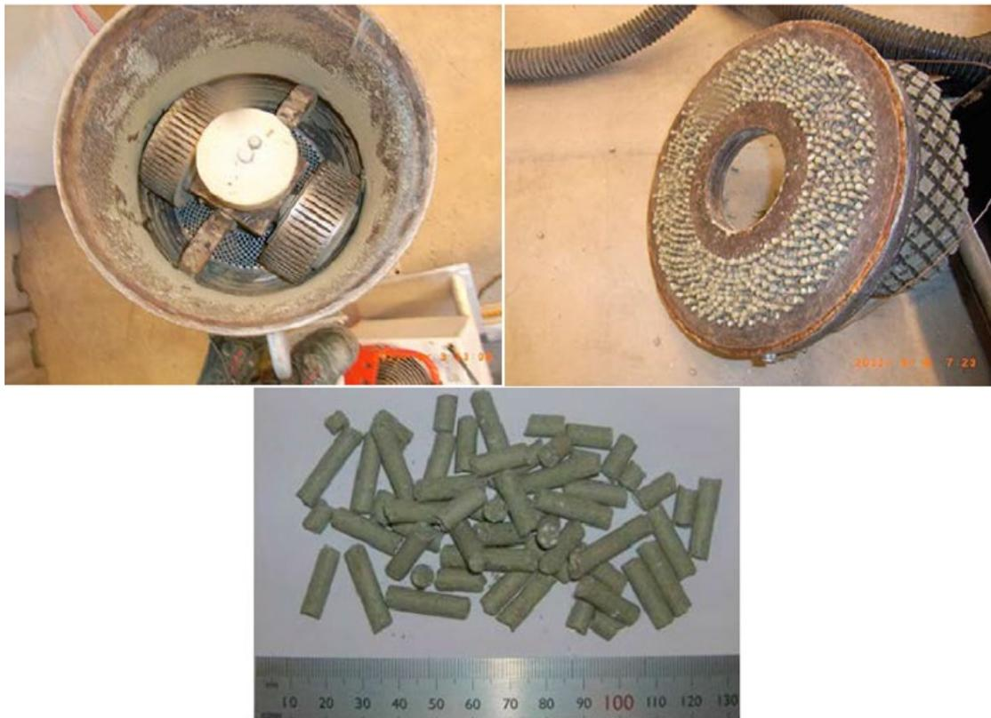
Figure 2-29 Extruded pellets composed of IBECO bentonite (Johnsson and Sandén 2013).
