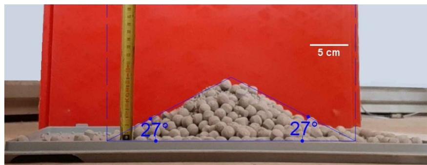
Figure 5-6 Photograph of experimental pellet pile formed by the optimum DEM GSD.
