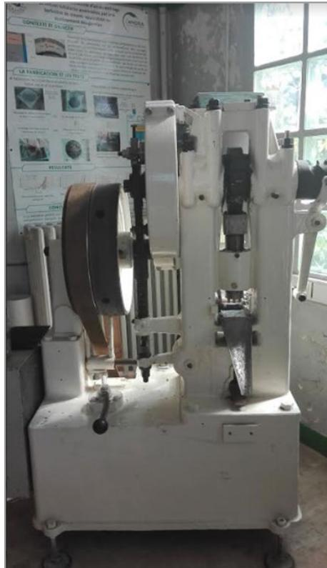
Figure A-1 Frogerais 1B tablet press machine used for the pellet fabrication.
