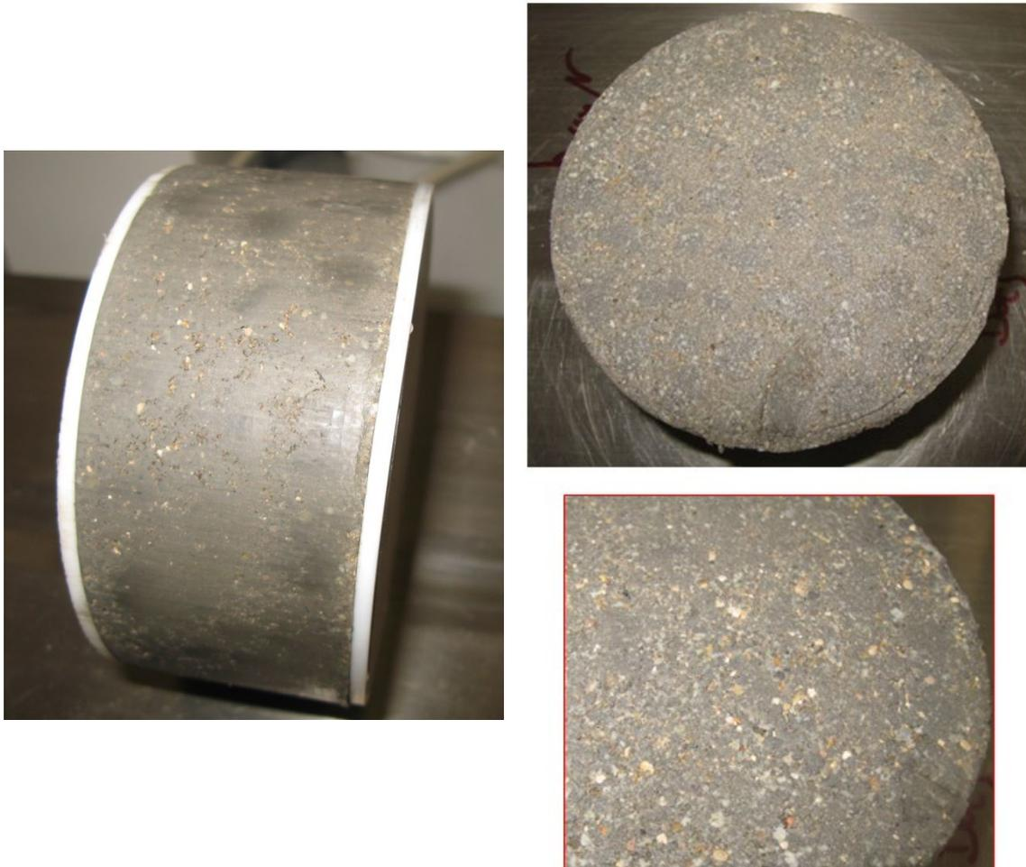
Figure 7-15 Specimens of Mixture 3 (16 mm, 10 mm, crushed pellets and sand) prepared at initial dry density of  $\rho_d = 1.60 \text{ Mg/m}^3$  (70P-15CP-15WGS) at the end of swelling pressure and permeability test ( $D=120 \text{ mm}/H=50 \text{ mm}$ ).
