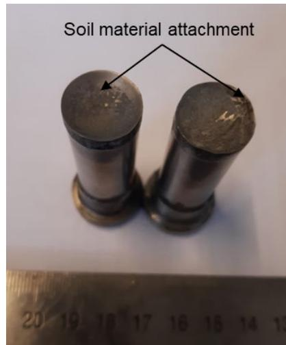
Figure 4-22 Observed soil attachment to the punch tool with the initial curvature.
