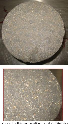
Figure 7-15 Specimens of Mixture 3 (16 mm, 10 mm, crushed pellets and sand) prepared at initial dry density of  $\rho_d = 1.60 \text{ Mg/m}^3$  (70P-15CP-15WGS) at the end of swelling pressure and permeability test (D=120 mm/H=50 mm)..
