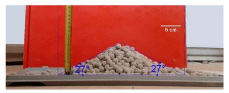
Figure 5-6 Photograph of experimental pellet pile formed by the optimum DEM GSD.
