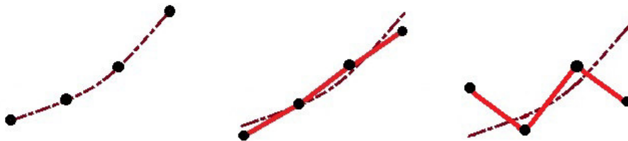
Figure 3.3: The presence of noise does not affect the signal patterns, as long as the variation is small compared to the curve’s slope.
