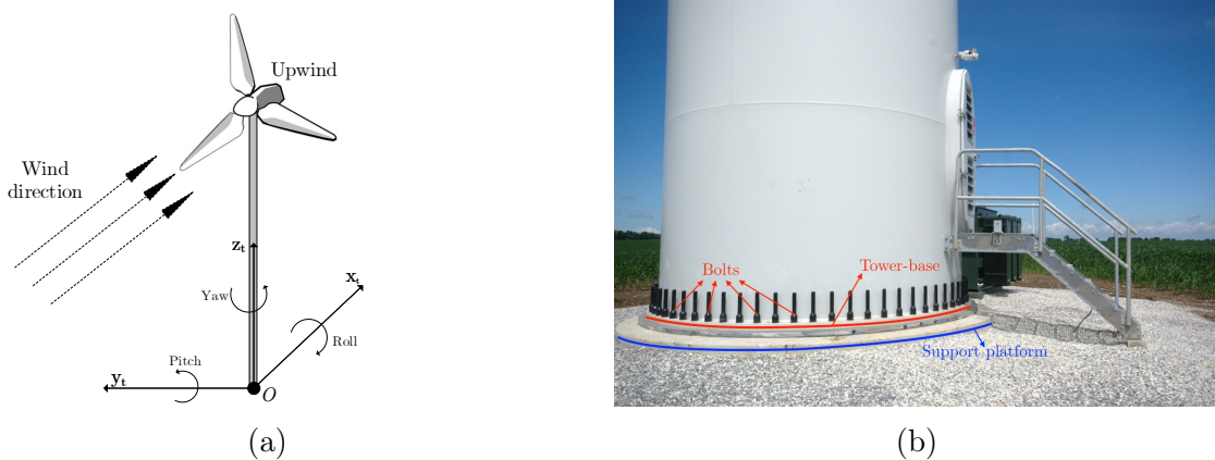
Figure 3.1: Tower-base coordinate system for upwind turbine: (a) a sketch; (b) an example of land-based wind turbine
