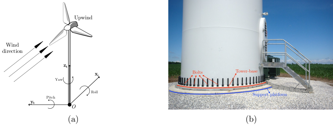
Figure E.1: Tower-base coordinate system for upwind turbine: (a) a sketch; (b) an example of land-based wind turbine 1
