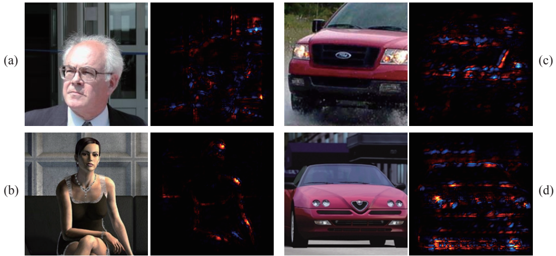
Figure 4.8: Heatmaps of four sample image patches. The top row corresponds to NIs, and the bottom row corresponds to CG images. Each group consists of the input image patch (left) and its heatmap (right). The red color in heatmaps stands for a large value, blue for a small value, and black for an intermediate value.
