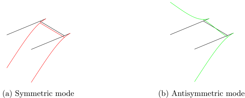
Figure 2.4: Mode shapes of two coupled cantilevers
