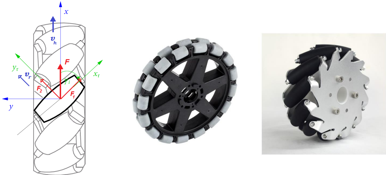
Figure 2.10 : Forces acting on the wheel and Omni wheels with rollers mounted at 90^\circ and rollers mounted at 45^\circ
