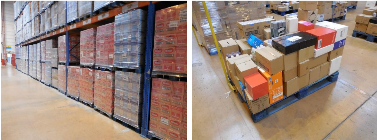
Figure 3.9 : Homogenous and Heterogenous Pallets
