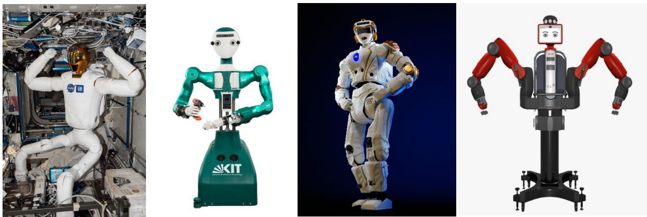
Figure 2.2 : Humanoids Robonaut 12 , Armar6 13 , Valkyrie 14 and Baxter
