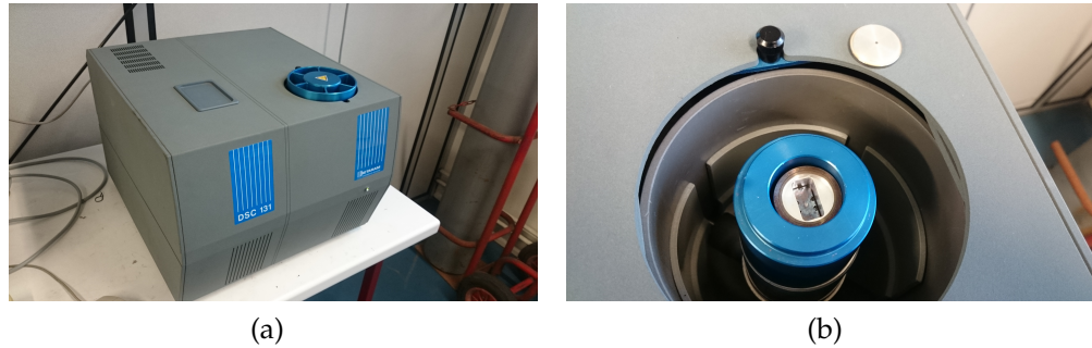
Figure 110: Pictures of the DSC device in IEMN (a) with a zoom on the crucible insert section (b)
