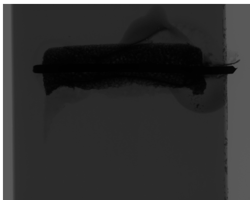
Figure 112: Microtomographie of 3D-C. The silver paste is visible on the top and the glass backing as well in the background but the Carbon foam is invisible.
