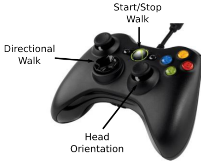
Figure A.4: The Xbox 360 controller used to control the robot walk.
