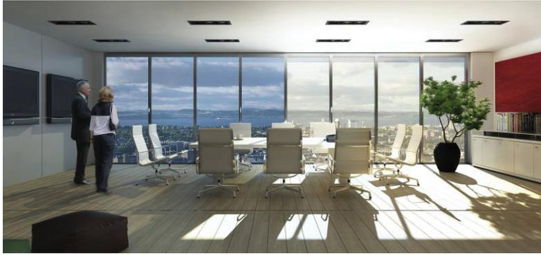
Figure 1. Illustration of a smart window proposed by the EControl-Glas GmbH. The left part is colored blue-gray and blocks some of the visible light and IR while the right part is colorless and transmissive to light [8].
