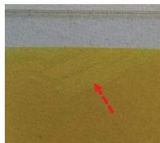
Figure 45. Surface scratch of V_2O_5 RF-metal thin film of 409 nm
