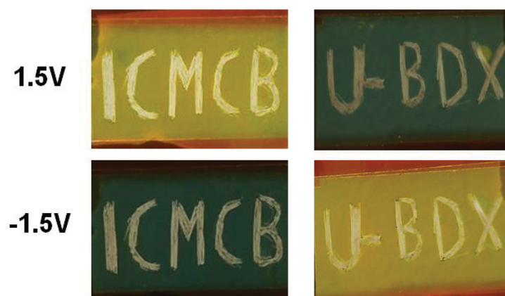
Figure 109. Color images at applied potential of EC device represented the labels for ICMCB and U-BDX. V_2O_5/LiTFSI-BMITFSI-40\% PMMA(70wt\%)-TiO_2(30wt\%)/V_2O_5
