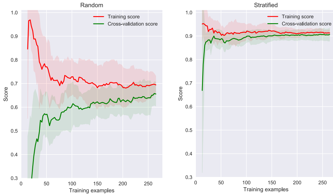
Figure 5. Learning curves of a naïve Bayes classifier. The graph compares the performance of a model on training and cross-validation data over an increasing number of samples. Random sampling dataset is contrasted with the stratified sampling dataset. The F-score metric was used to quantify the classification performance.
