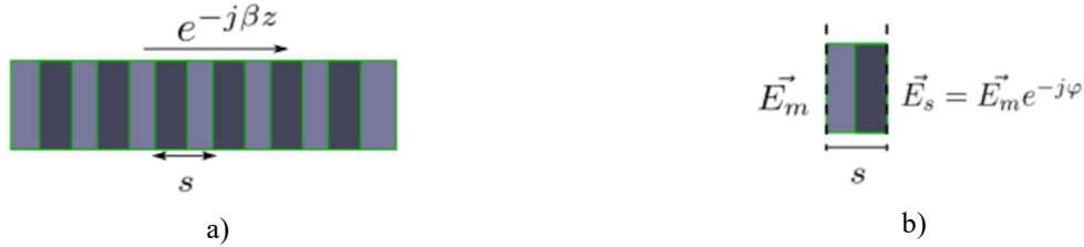
Figure 4-4. Principle of the eigen-mode simulation: a) periodic waveguide and b) equivalent resonant unit-cell [1].
