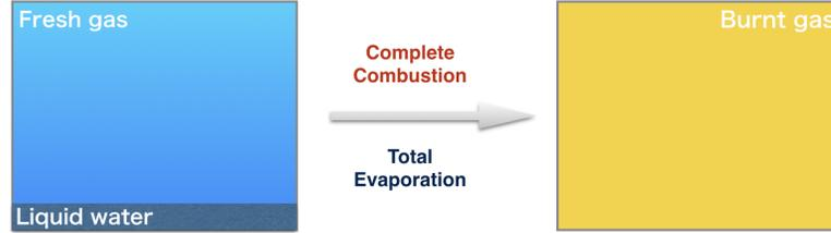
Figure 2.1: Lumped-parameter study: equilibrium solution of the simplified system
