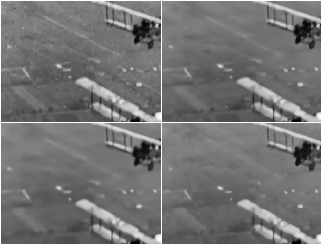
Figure 6.9: Blind denoising better preserves details than methods for a predefined noise. From top to bottom, left to right: original, blind denoising, denoising with the pre-trained network and VBM3D with hand-tuned noise parameter.
