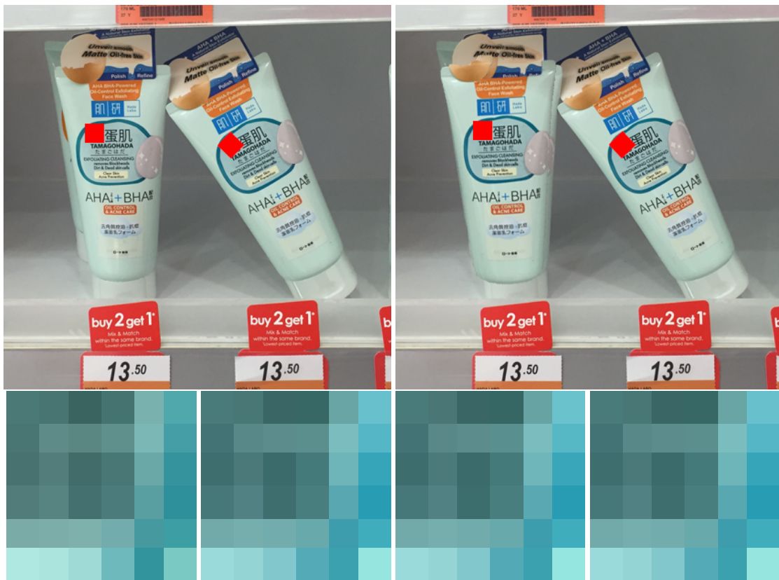
Figure 11: On the left image the two objects are similar but not digital copies of each other. On the right, one is a digital copy of the other. The patches shown below each respective image correspond to the red squares in the images. They show that a difference is visible at this level and therefore the descriptors can be discriminated. This is why the detection method can discard genuinely similar objects.
