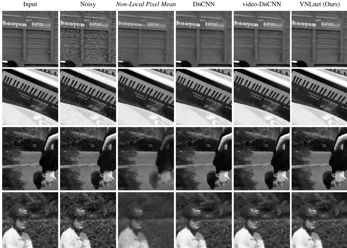
Figure 5.6: Example of denoised result for Non-Local Pixel Mean , DnCNN, video-DnCNN (see Section 5.4.3) and VNLnet, for AWGN with \sigma = 20 . The four crops highlight the results on frames feature various kinds of motion. The videos are part of the DAVIS dataset. Non-Local Pixel Mean corresponds to the average of the output of the non-local patch search.
