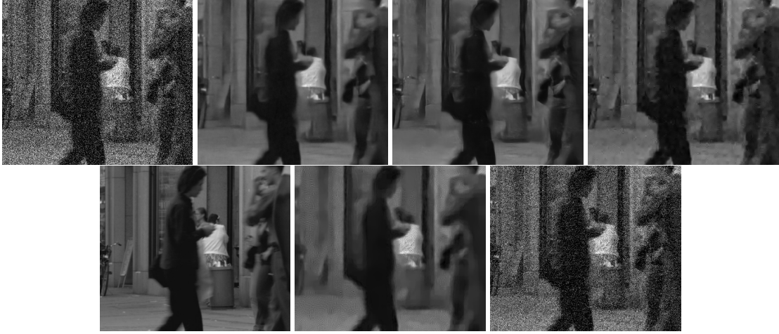
Figure 6.5: Example of denoising of an image corrupted by a Gaussian noise of standard deviation \sigma = 50 . The fine-tuned network doesn't produce any visible artifact, the results are comparable to a DnCNN trained for this particular type of noise. From left to right, top to bottom: Noisy, fine-tuned, DnCNN trained for a Gaussian noise with \sigma = 50 , VBM3D, ground truth, noise clinic, DnCNN trained for a Gaussian noise with \sigma = 25 .
