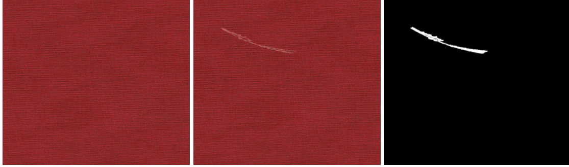
Figure 9.5: A ground truth (on the right) for anomaly detection has been generated by introducing an anomaly in a RPN [GGM11b] texture (on the left), which is anomaly free. The detection is then done on the result (in the middle).
