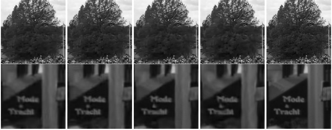
Figure 3.2: Denoising results when the sequence is corrupted by noise of standard deviation 30. From left to right: Denoising using NL-Kalman, NL-Kalman with the oracle optical flow, VBM3D, VBM4D and the original. From top to bottom: Crop from the sequence crowd_run and pedestrian_area . Overall the proposed method preserves more details as can be seen both in the tree and in the text. Results best viewed zoomed.
