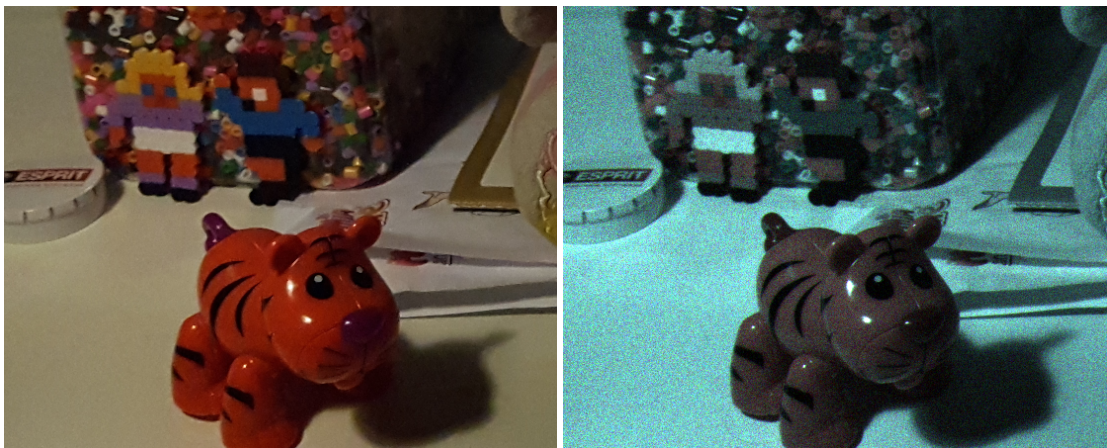
Figure 1: While the final output of a Samsung Galaxy S7 doesn't show apparent noise (left), the RAW image seen by the sensor is actually very noisy (right). The final output is obtained thanks to a complex processing that applies denosing as one of its step.
