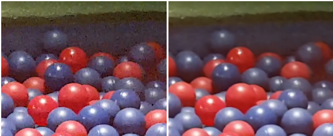
Figure 6.11: Example of denoised image (right) coming from a mobile phone (left). The results is more natural and pleasing to the eye as it doesn't have all these ugly artifacts.
