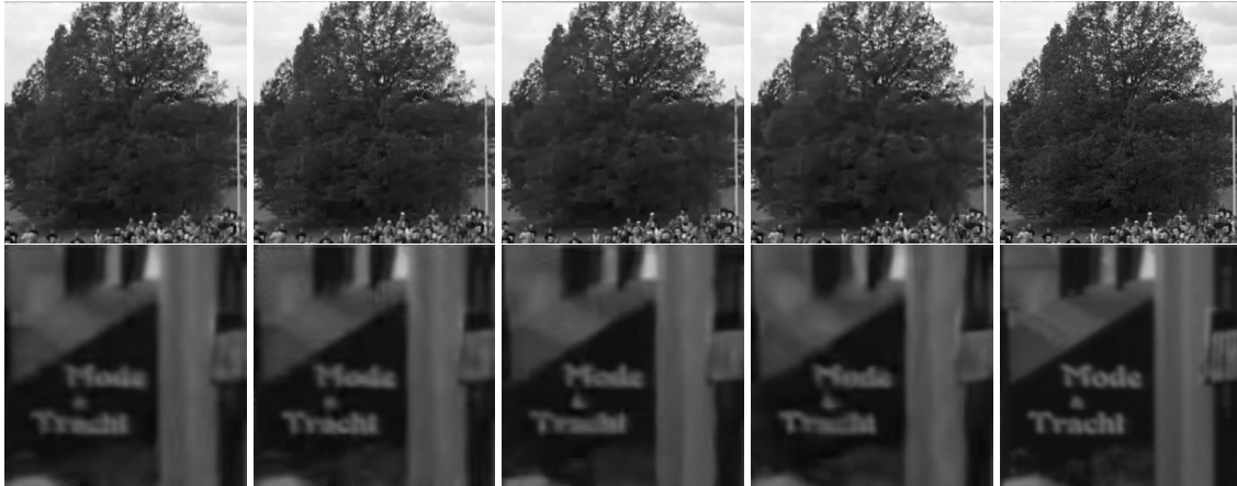
Figure 4: Denoising results when the sequence is corrupted by noise of standard deviation 30. From left to right: Denoising using NL-Kalman, NL-Kalman with an oracle optical flow, VBM3D, VBM4D and the original frame. From top to bottom: Crop from the sequence crowd_run and pedestrian_area . Overall the proposed method preserves more details as it can be seen both in the tree and in the text. Results best viewed zoomed.
