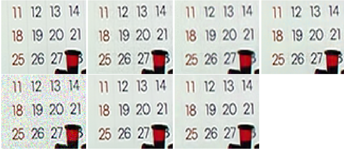
Figure 2.5: Results of denoising for mobile (zoom on frame 37, noise 20). Top: ground truth, NL-Bayes local, BM3D local, VBM4D; bottom: Noisy, NL-Bayes global and BM3D mix.
