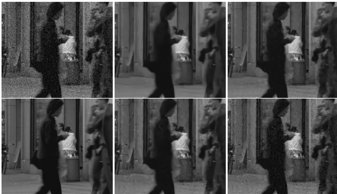
Figure 6.4: Example of denoising of an image corrupted by a JPEG compressed Gaussian noise. The fine-tuned network doesn't produce any visible artifacts, contrary to the original DnCNN used for the fine-tuning process. From left to right, top to bottom: Noisy, fine-tuned, VBM3D, ground truth, DnCNN trained for a Gaussian noise, noise clinic.
