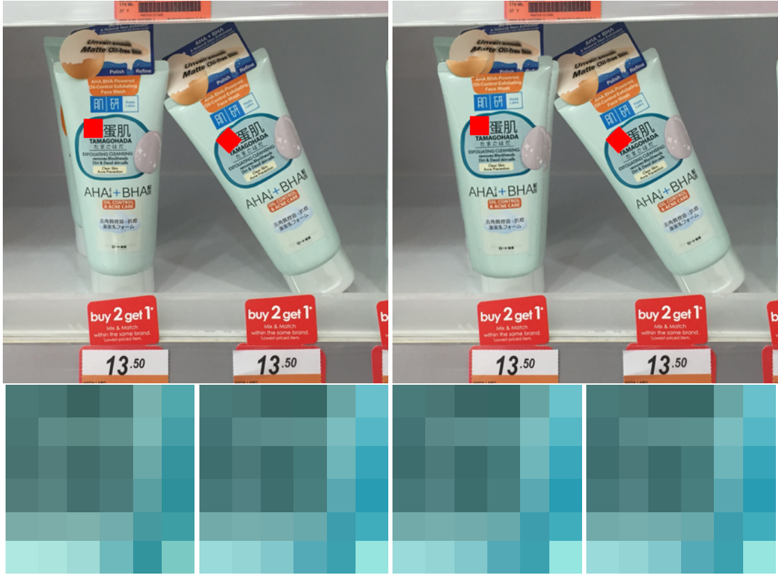
Figure 12.1: On the left image the two objects are similar but not digital copies of each other. On the right, one is a digital copy of the other. The patches shown below each respective image correspond to the red dots in the images. They show that a difference is visible at this level and therefore the descriptors can be discriminated. This is why the detection method can discard genuinely similar objects.
