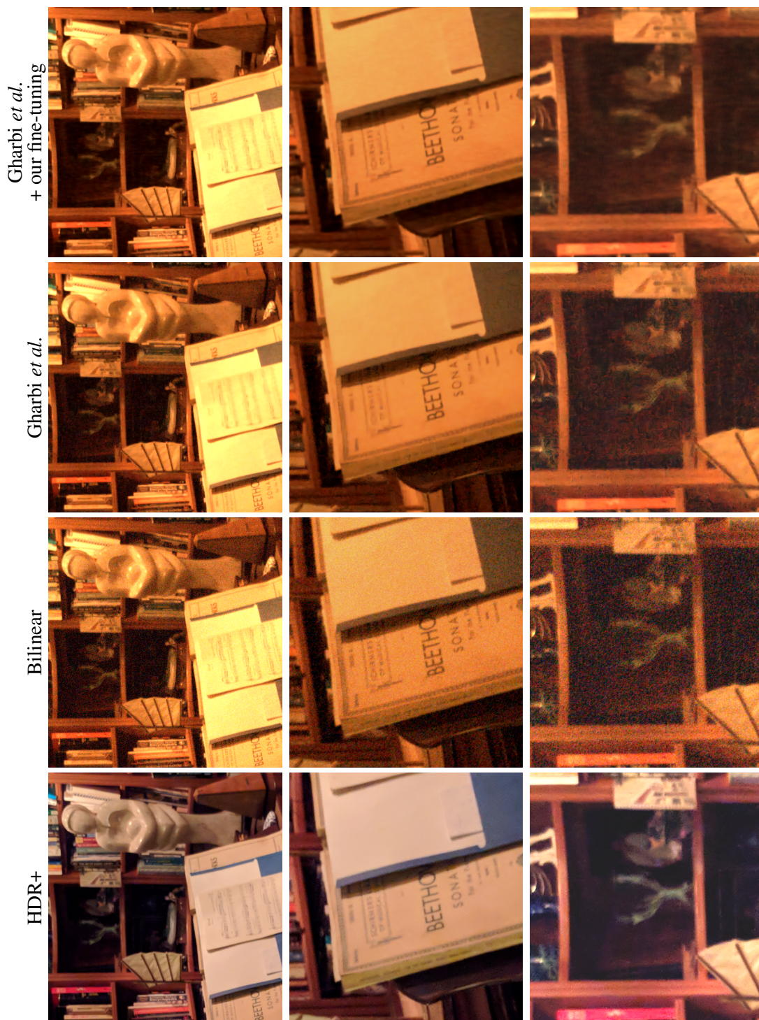
Figure 8.14: Experiment on a real burst. Left to right: The result of the HDR+ pipeline [HSG + 16], bilinear interpolation, Gharbi et al. [GCPD16], and Gharbi et al. [GCPD16] with our fine-tuning. Contrast in dark regions was enhanced for all methods. Note that the HDR+ pipeline includes color balance as well as sharpening. It also uses all the images of the burst to produce the result (all other methods use only the reference frame). Figure best visualized zoomed in on a computer.
