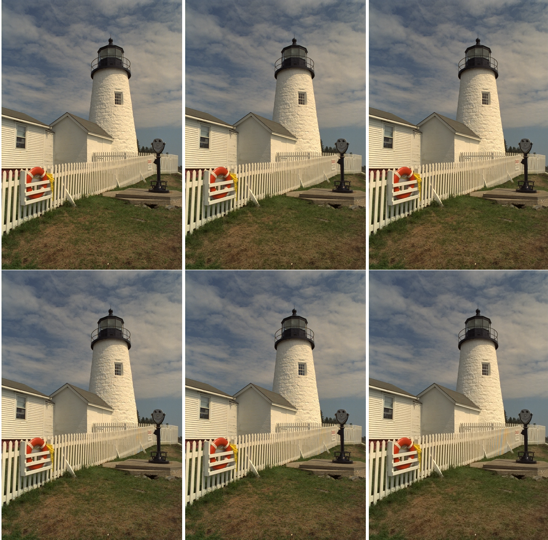
Figure 7.6: From top-left to bottom-right: Original, Gharbi et al. [GCPD16], Tan et al. [TZZZ17], MLRI [KMT014], ARI [MKTO15], Getreuer [Get12]. All demosaicing methods shown here perform well overall, with no visible strong artifacts. Yet a moiré artifact appears in the fence for some of the methods.
