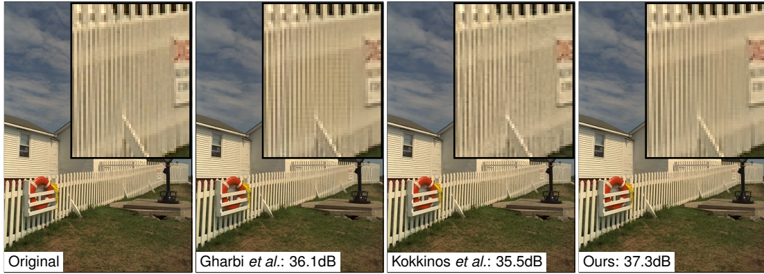
Figure 8.1: Using a burst, our fine-tuning (starting from the network from Gharbi et al. [GCPD16]) is able to not only denoise well ( \sigma = 5 ) but also doesn't show any artifacts like zipper or moire in the difficult regions. Best visualized on a screen.
