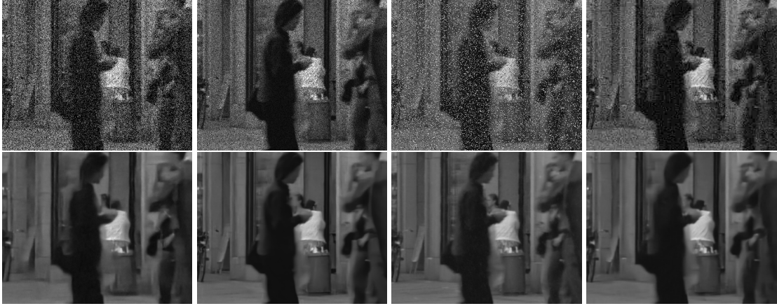
Figure 6.1: From the same starting point and only using the video, our fine-tuned network is able to denoise different noises without any artifact. The top images are the noisy and the bottom ones the denoised. From left to right: Gaussian noise, Poisson type noise, salt and pepper type noise and JPEG compressed Gaussian noise.
