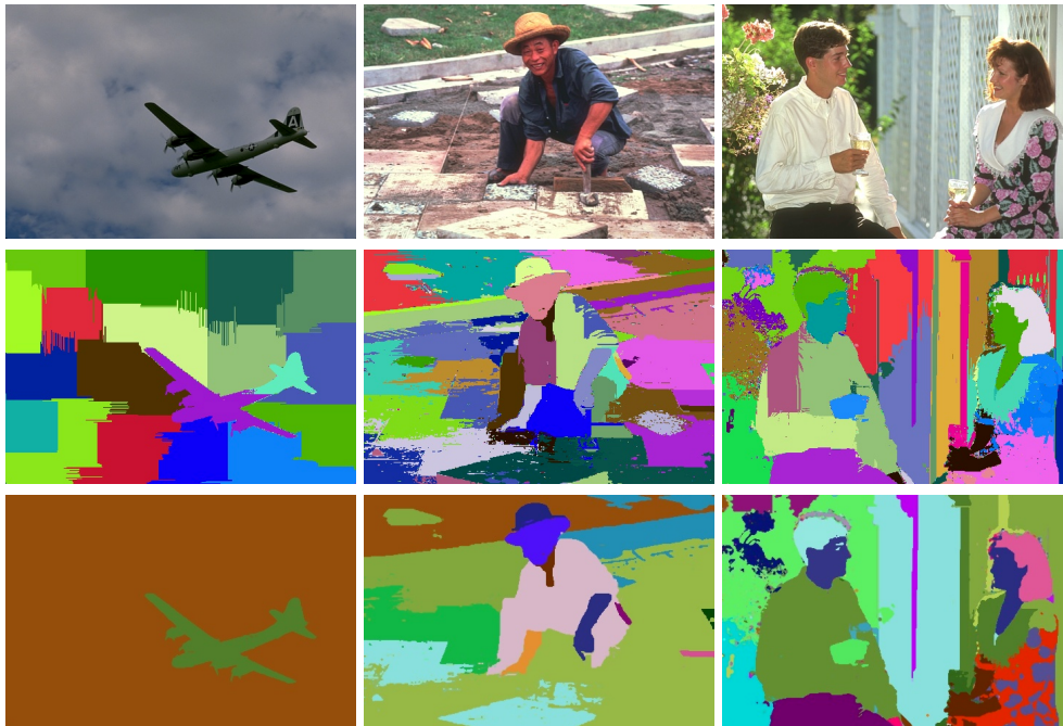
FIGURE 4.3: Image segmentation results: Top : Original images. Middle : after the execution of the Louvain method. Bottom : after the merging of homogeneous regions using both Mean and Standard deviation feature and the ARA algorithm.
