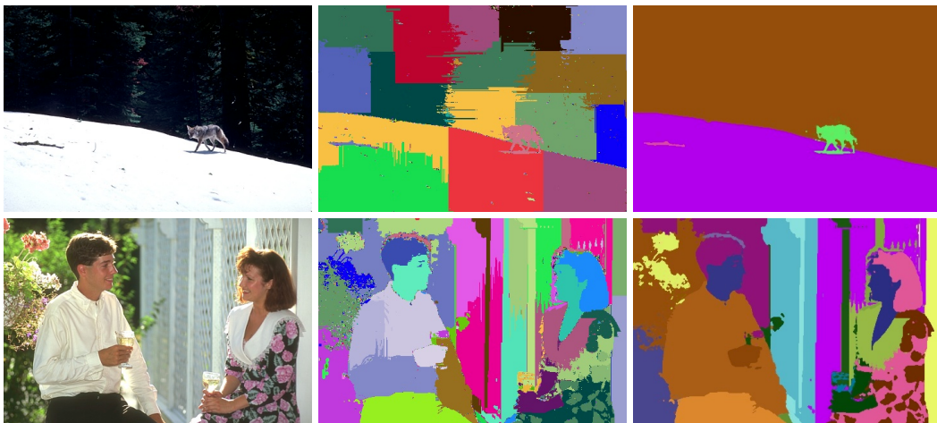
FIGURE 4.7: Image segmentation results: Left: Original images. Middle: after the execution of the Louvain method. Right: after the merging of homogeneous regions using both reduced histogram of colors and the ARA algorithm (Nguyen, Coustaty, and Guillaume, 2018b)
