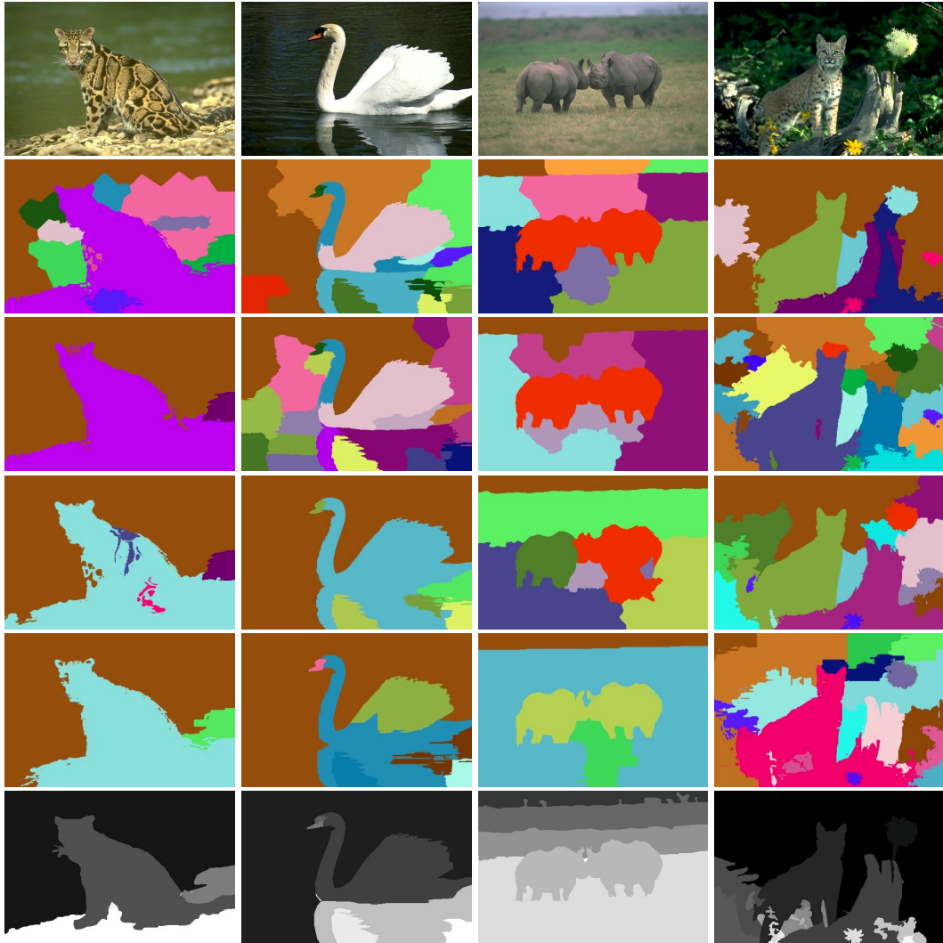
FIGURE 5.2: Qualitative evaluation of results using Best pattern (Pattern A) on BSDS 500 dataset. First line : Original images, Second line : Results of using RH feature, Third line : Results of using MeanSD feature, Fourth line : Results of using HOGMeanSD feature, Fifth line : Results of using BHMF feature, Sixth line : Ground-truth.
