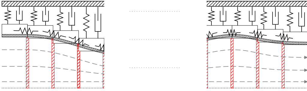
Figure 3.4 – Finite-dimensional formulation of the fluid-structure system. MSD-based description of the structure motion. Fluid dynamics description based on nodes (red) and incompressible fluid sections.
