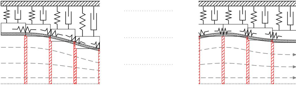
Figure 3.4 – Finite-dimensional formulation of the fluid-structure system. MSD-based description of the structure motion. Fluid dynamics description based on nodes (red) and incompressible fluid sections.
