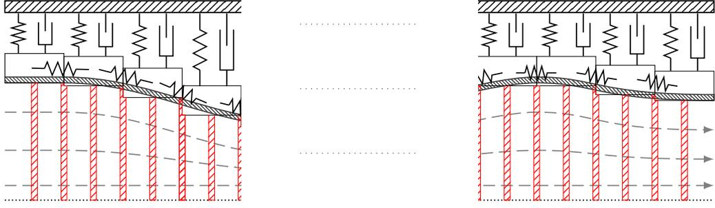
Figure 3.5 – Finite-dimensional formulation of the fluid-structure system with  $n_f \neq n_s$ .
