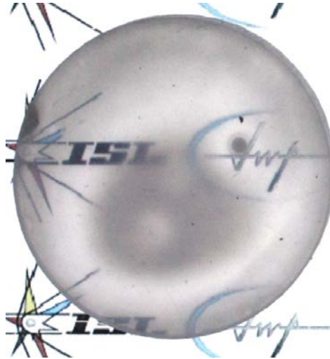
Figure IV.7: SPS sintered specimen obtained from the 3 layers of powder (0.47 wt% / 0.235 wt% / 0 wt%). (30 mm diameter, thickness: 4.3 mm).
