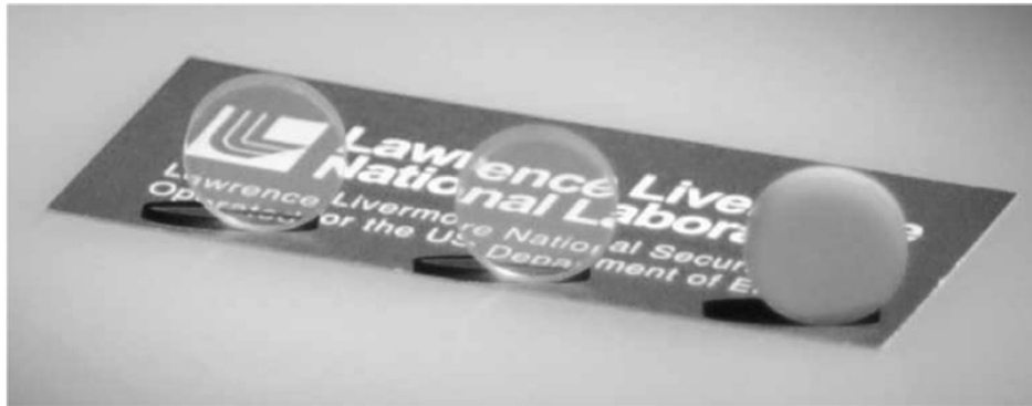
Figure I.24: Polycrystalline multilayer ceramic obtained by dry pressing method. Effect of HIP treatment under 200 MPa was shown on sintered ceramics (from left to right): 1750 °C 4h, 1650 °C 4h and as-sintered (9.5 mm diameter, 1.5 mm thick) from [143].
