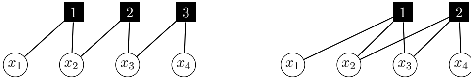
Figure 1.2: A graphical representation of a Markov chain of order one (left) and of order two (right).
