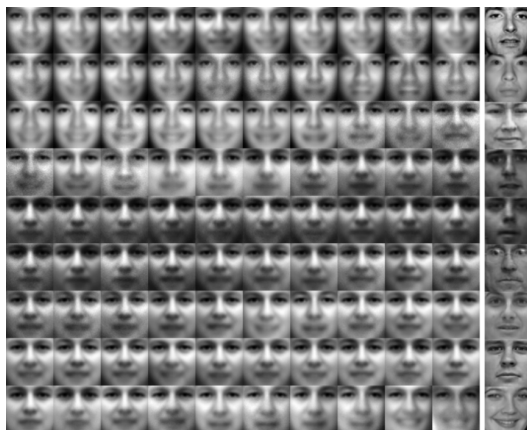
Figure 2.2: Synthetic samples generated by running the Markov chain of a GSN. The image from the training set closest to the final synthetic image in each row is shown in the final column. Figure taken from [Bengio et al. 2014].
