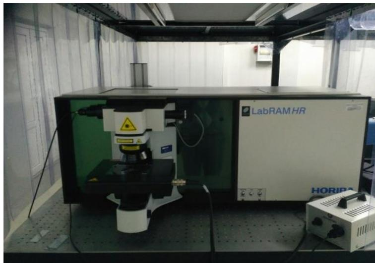
*Figure 5 Labram HR Raman spectrometer installed in MONARIS Laboratory*
