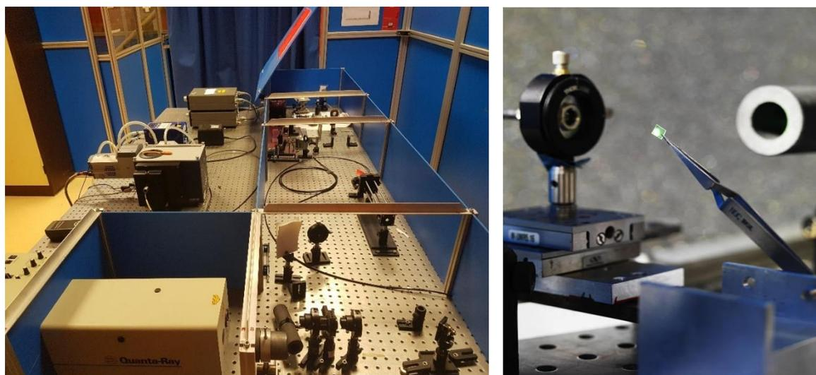
Figure 2 Experimental setup for the photoluminescence measurements ( $\lambda_{ext} = 266, 355$  and  $532$  nm (LSI)).
