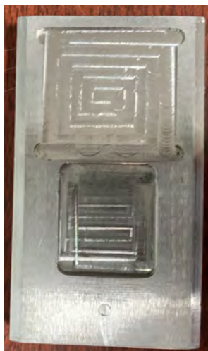
Figure 2.5 Stainless steel sample holder.
