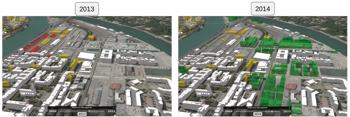
Figure 3.11.: Screenshots showing the evolution of a district of the city of Lyon (in 2013 on the left side and in 2014 on the right side) visualized in UD-Viz and using 3D Tiles extended with 3DTiles_temporal .
