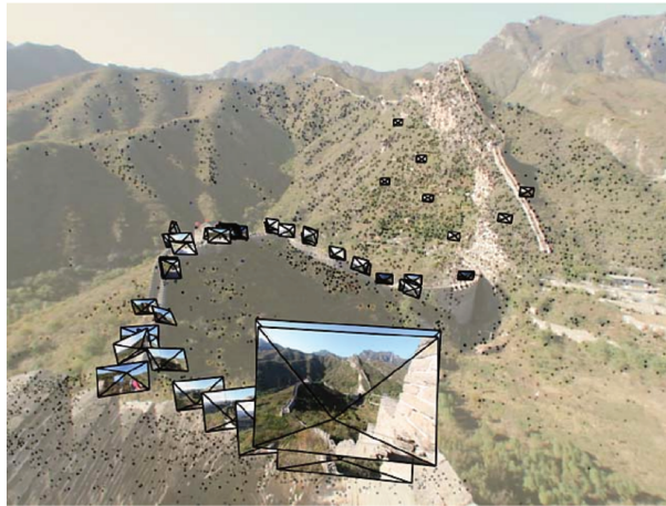
Figure 2.11.: A set of pictures calibrated over a 3D model. Image extracted from [Sna+06].
