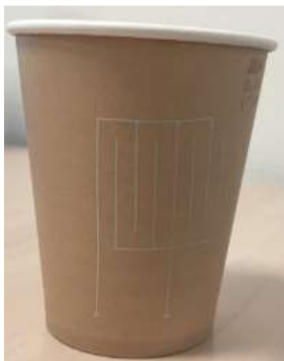
Figure 102: Printed circuit on paper cup with adjusted parameters
