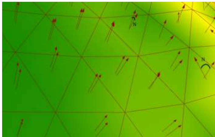
Figure 46: Deviation between triangulated and smoothed faces normal
