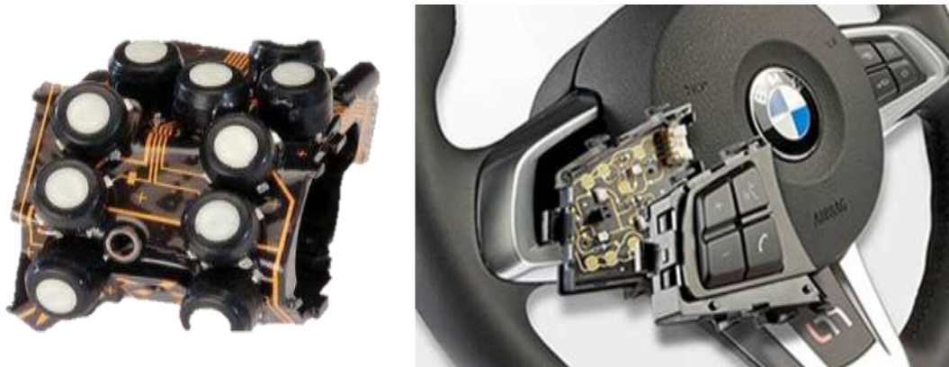
Figure 22: Plastronic motorcycle handles and steering wheel BMW
