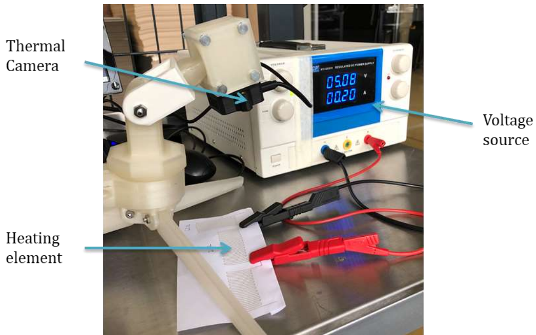
Figure 121: Experimental set-up for temperature measurements
