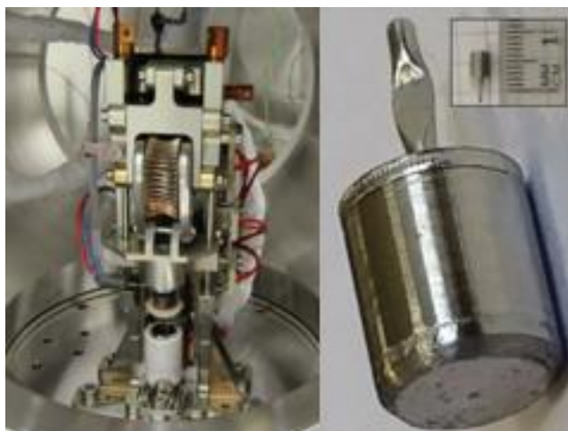
Figure 1-13 Tapping station with its oven (left) and derivatization capsule (right).
