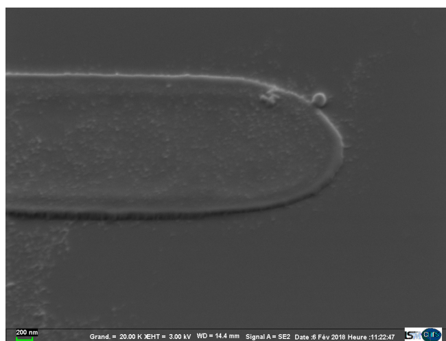
Figure 6-8. SEM image of segmented line in Fig 6-7 (side view 45°)
