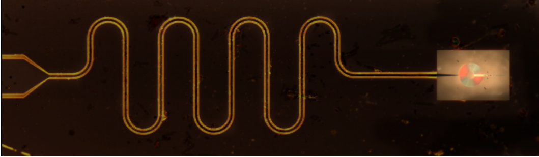
Figure 3.10: Optical image of the whole 3 mm \times 10 mm chip, showing the impedance adaptation resonator (meanders in the middle) and the bonding pad on the left (taken from [35]).
