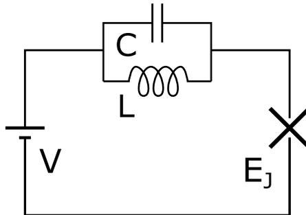
Figure 1.7: A  $LC$  resonator hosting a single mode of radiation is put in series with a dc bias source and a JJ. The two dipoles are coupled: inelastic tunneling across the junction can be prompted by the voltage fluctuations in the resonator. At the same time the tunnel current through the junction is directly injected into the oscillator, creating excitations in the mode.
