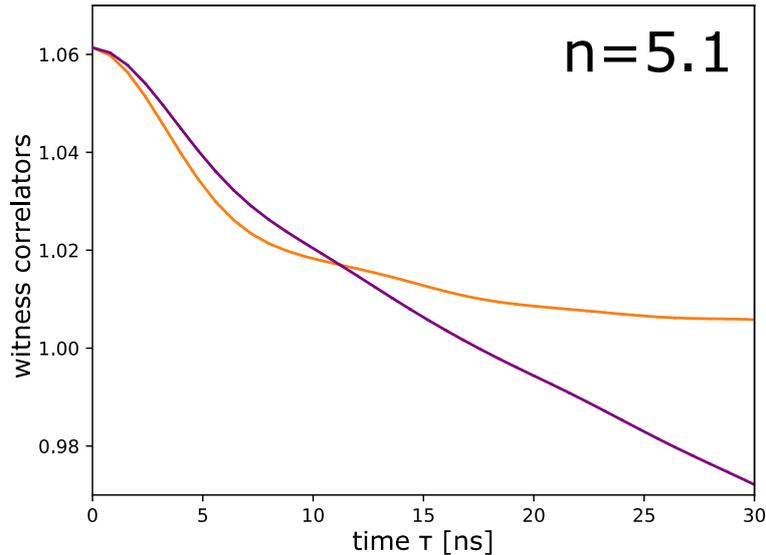
Figure 4.53: Witness correlators measured at  $\bar{n} = 5.1$  with narrower filters. Parasitic oscillations in the correlation functions have been reduced. The witness inequality (4.41) is violated by  $13 \sigma$ .
