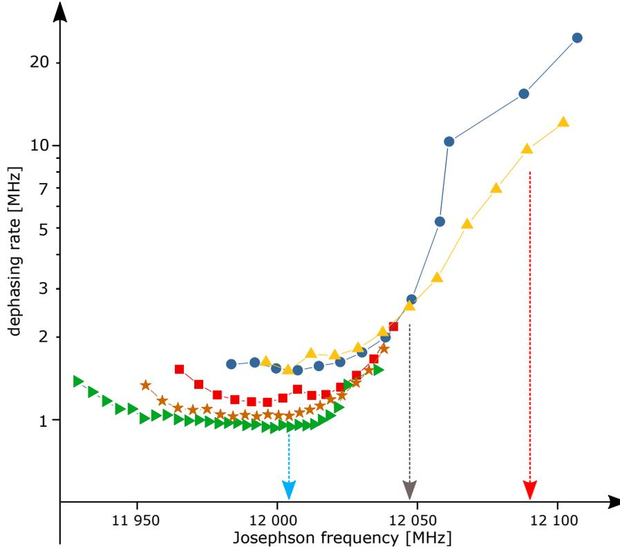
Figure 4.42: Dephasing rate  $\sigma_\omega/2\pi$  of the phase correlator for different values of  $\beta$ , as a function of the Josephson frequency. The red arrow indicates the bias voltage used in the preliminary experiment, which lies in the heating regime. The grey arrow indicates the bias neutral point  $\omega_J = \omega_a + \omega_b$ . The light blue arrow points to the optimal cooling point at  $\Delta = -\frac{\kappa_a + \kappa_b}{2\sqrt{3}}$ .
