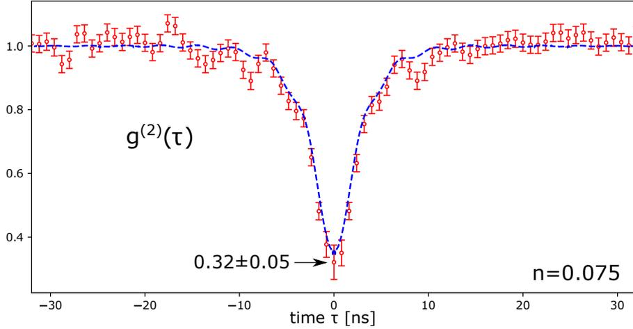
Figure 1.10: Second order coherence function of the photons emitted by the strong-coupling sample at low occupation number  $n = 0.075$  of the resonator. The value  $g^{(2)}(0) = 0.32$  proves the sub-Poissonian statistics of the photon, at an emission rate  $\Gamma \simeq 60$  Mphotons/s.
