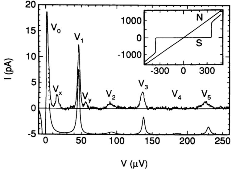
Figure 1.5: Experimental  $I(V)$  measured in [32]. A dc current is measured below the gap voltage  $2\Delta/2$ , due to inelastic Cooper pair tunneling processes. Each peak at bias voltage  $V_i$  is associated to the emission of light in a resonance of the environment at frequency  $2eV_i/\hbar\omega$ , in processes where one photon is created for each transferred Cooper pair.
