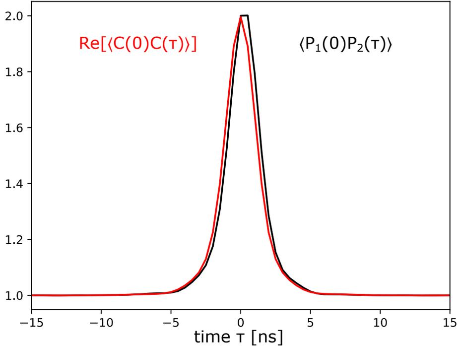
Figure 3.52: Second order coherence functions computed either from (3.87) (black curve) or (3.88) (red curve).
