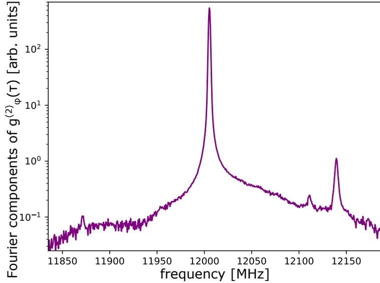
Figure 4.52: Fourier transform of the phase correlator at  $\bar{n} = 9.25$ . In addition to the main Gaussian peak at 12.005 GHz due to the direct emission of entangled photons, Stokes and Anti-Stokes processes are visible at 11.87 GHz and 12.14 GHz respectively, as well as a single Anti-Stokes peak at 12.11 GHz.
