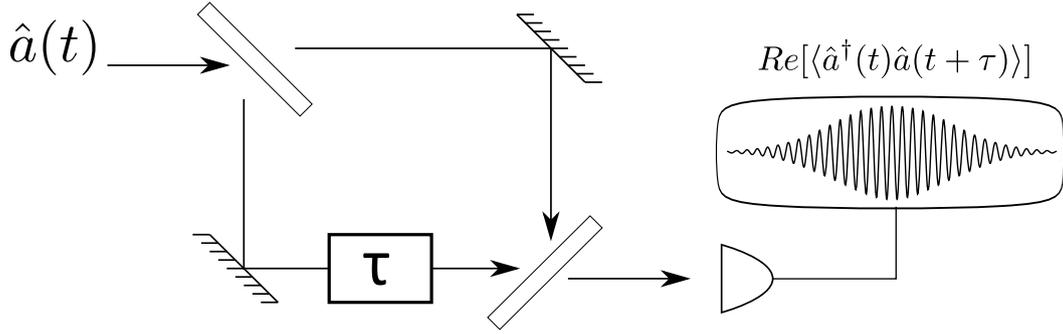
Figure 3.15: Mach-Zehnder interferometer. The incoming field  $\hat{a}(t)$  is split onto two different paths by a beamsplitter. The traversal time of the two paths differ by a certain delay  $\tau$ . When recombined the two beams interfere, with a fringe contrast proportional to  $Re[g^{(1)}(\tau)]$ .
