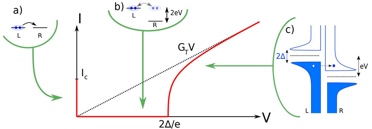
Figure 2.3: The three branches of the  $I(V)$  of a superconducting tunnel junction: a) At zero bias, the supercurrent results from the elastic transfer of Cooper pairs from one BCS condensate to the other. b) At  $V \neq 0$ , the irreversible transfer of Cooper pairs is prohibited:  $\langle I \rangle = 0$ . c) Above the gap voltage, normal quasiparticles can tunnel, as in a normal junction.
