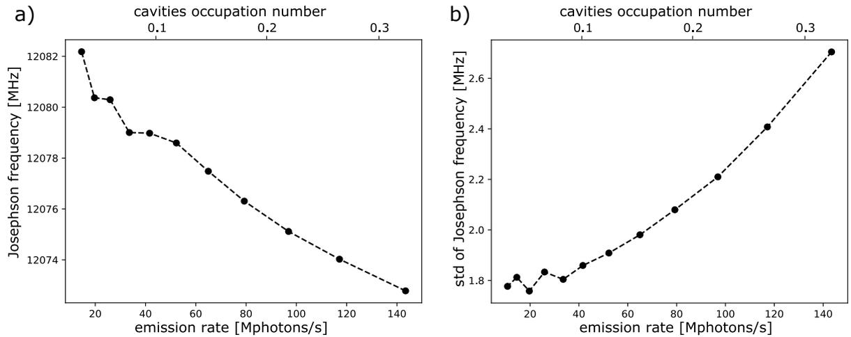
Figure 4.41: a) Josephson frequency as a function of the emission rate  $\Gamma$  and the occupation number  $\bar{n}$ . b) Standard deviation of the Josephson frequency  $\sigma_\omega/2\pi$ , extracted from the Gaussian fits of figure 4.40.
