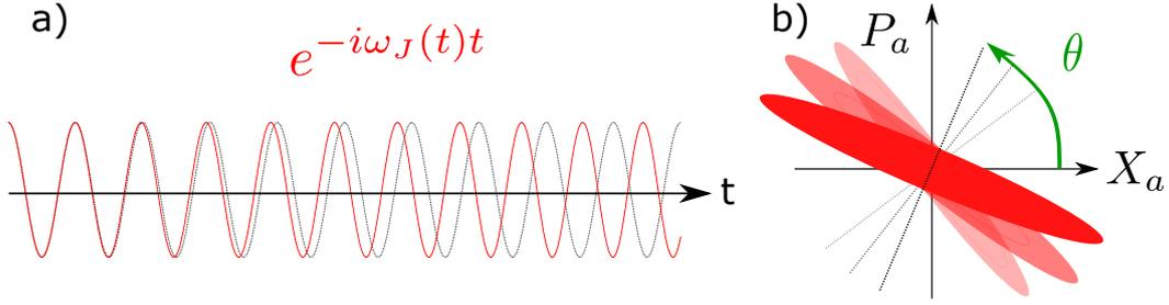
Figure 4.4: a) Due to thermal voltage noise on the junction, the Josephson frequency  $\omega_J$  fluctuates randomly. The  $e^{-i\omega_J(t)t}$  driving term (real part in red) in the squeezing Hamiltonian (4.8) dephases slowly with respect to a pure sinusoidal tone (dashed grey). b) The squeezing angle  $\theta$  drifts randomly with time, making a direct measurement of quantum squeezing impossible.
