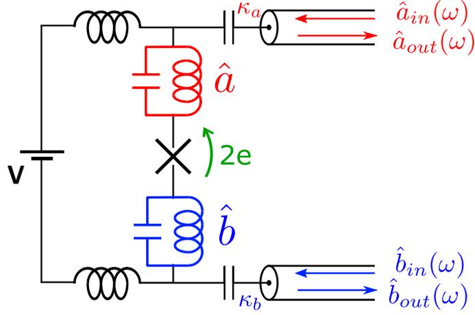
Figure 4.11: Input-output model for the two-resonator experiment. The  $a$  ( $b$ ) cavity is driven by the effective Hamiltonian (4.16), is subject to incoming vacuum noise from the transmission line at frequency  $\omega_a$  ( $\omega_b$ ), and re-emits photons in the line.
