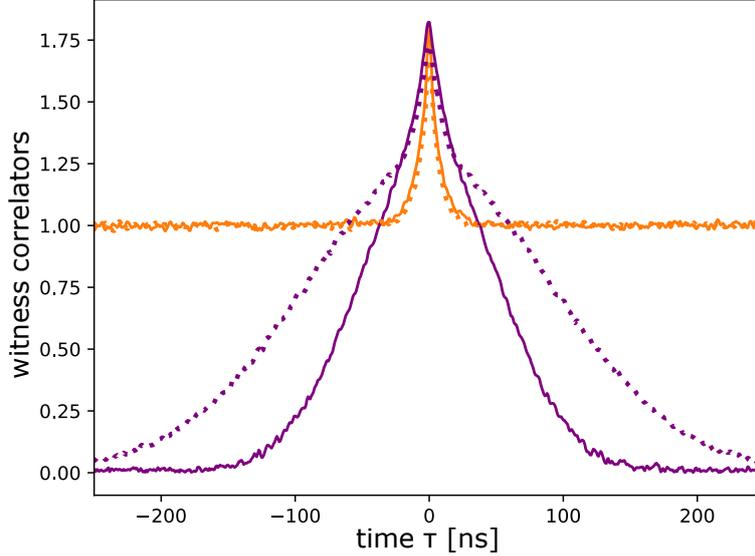
Figure 4.49: Entanglement correlators measured at  $\bar{n} = 1.0$  both at the neutral point (full lines) and in the cooling regime (dashed lines). The Gaussian decay rate of the phase correlator is reduced in the cooling regime, yielding a longer entanglement time.
