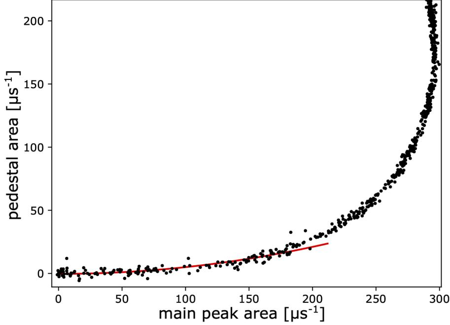
Figure 3.46: Contribution of the pedestal to the emission rate, as a function of the main peak area (in black), with quadratic fit (red), fitted for  $\Gamma < 200$  MHz. As for low emission rates the main peak scales as  $E_J^2$ , this indicates that the pedestal area scales as  $E_J^4$ .
