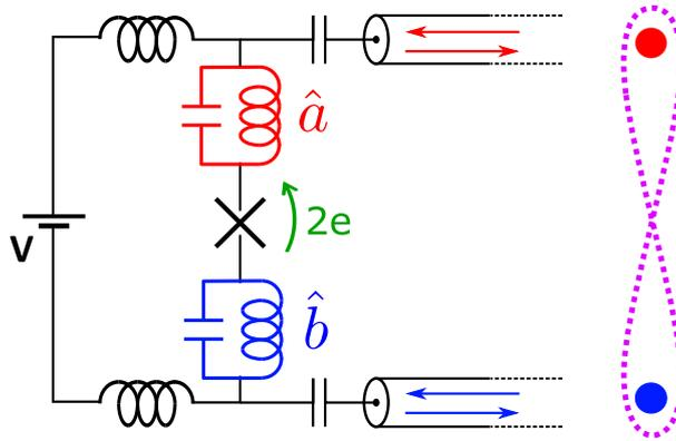
Figure 1.11: Two resonators at frequencies  $\omega_a, \omega_b$  are connected to a dc-biased JJ. When  $2eV = \hbar\omega_a + \hbar\omega_b$ , entangled photon pairs are created upon the tunneling of Cooper pairs .
