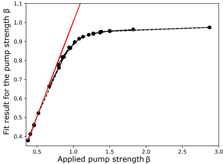
Figure 4.29: Results of the fit of 25 emission spectra, with the pump strength  $\beta$  varying from 0.41 to 2.87 and various values of the detuning  $\Delta$ . The fitted pump strength (black dots) agrees well with the true  $\beta$  (red line) at low driving, but disagrees for strong driving.
