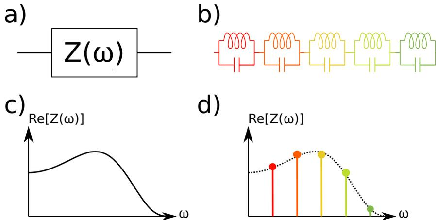
Figure 2.6: a) A linear impedance  $Z(\omega)$  models the environment of the junction. b) It can be replaced in the circuit by a collection of  $LC$  modes of various frequencies and impedances. c) The real part of  $Z(\omega)$  has some frequency dependence. d) Real part of the impedance of the  $LC$  modes. An infinite number of  $LC$ s can model any  $Z(\omega)$ .
