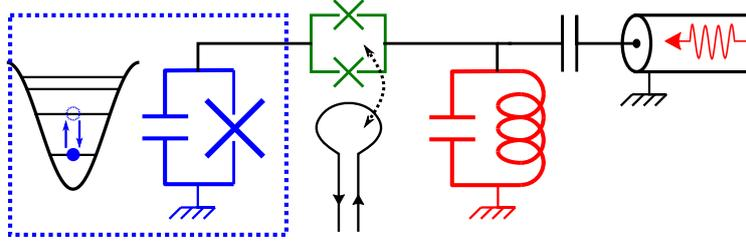
Figure 1.2: Example of a superconducting circuit where various JJs (crosses) are used to manipulate quantum information. A JJ in parallel with a capacitance (in blue) forms an anharmonic oscillator. This qubit can be selectively coupled to an electrical resonator (in red) through a Superconducting QUantum Interference Device (in green), whose admittance can be quickly varied by threading a magnetic flux through the loop (green arrow).
