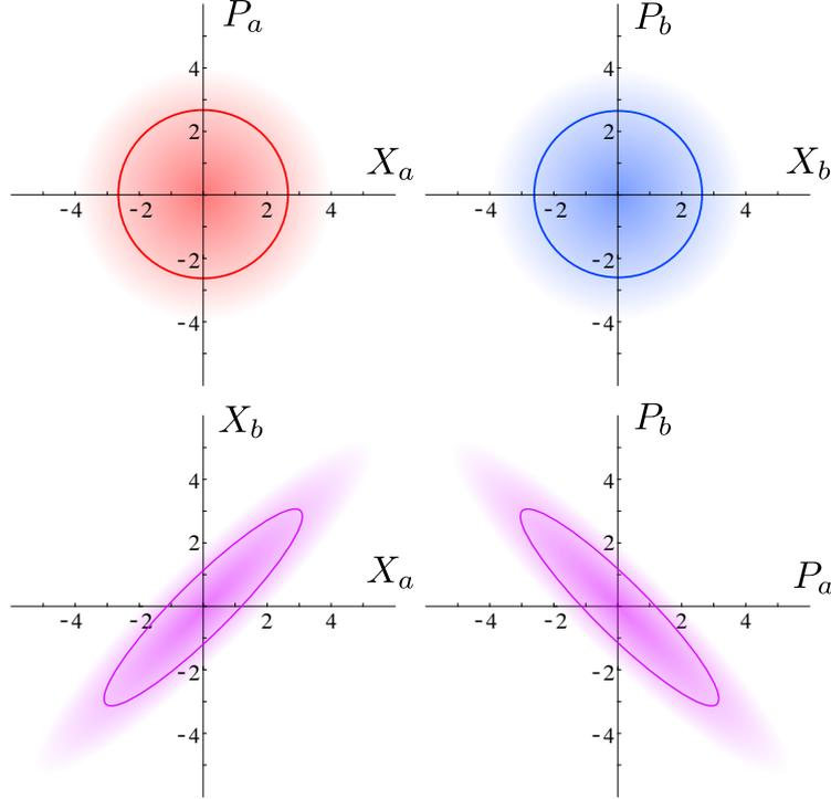
Figure 4.5: Wavefunctions of a two-mode squeezed vacuum (TMSV) with squeezing angle  $\theta = 0$ , in different pairs of quadrature bases. In the  $X_a, P_a$  basis, the TMSV shows no preferential orientation, and more noise than the vacuum state (not pictured). Same goes in the  $X_b, P_b$  basis. Wavefunctions in composite bases show correlations between  $X_a$  and  $X_b$ , and anti-correlations between  $P_a$  and  $P_b$ .
