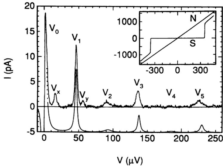
Figure 2.12: Experimental  $I(V)$  of the sample, with the  $P(E)$  prediction shifted down by 5 pA for clarity. Inset: the  $I(V)$  in a wider voltage range and a much bigger current scale, measured with the junction either in the superconducting state ( $S$ ), or driven normal by the application of a 1 T static magnetic field ( $N$ ). Figure taken from Holst et al., PRL 1994.
