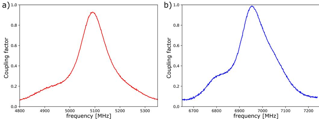
Figure 4.21: Emission spectra around  $\omega_a$  (panel a) and  $\omega_b$  (panel b) in shotnoise regime yield the microwave coupling factor between the junction and the resonators, as defined by (4.124).
