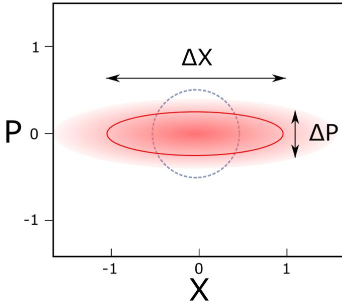
Figure 4.2: Probability distribution for the quadratures of a quantum squeezed state (red cloud). The standard deviation (red line) of  $X/P$  is larger/smaller than for the vacuum state (dashed gray).
