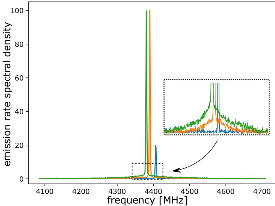
Figure 3.44: Spectra taken at three increasing values of  $E_J$  (blue, orange and green curves). The inset shows a zoom-in on the peak's pedestal, which keep increasing with  $E_J$  while the peak amplitude saturates.
