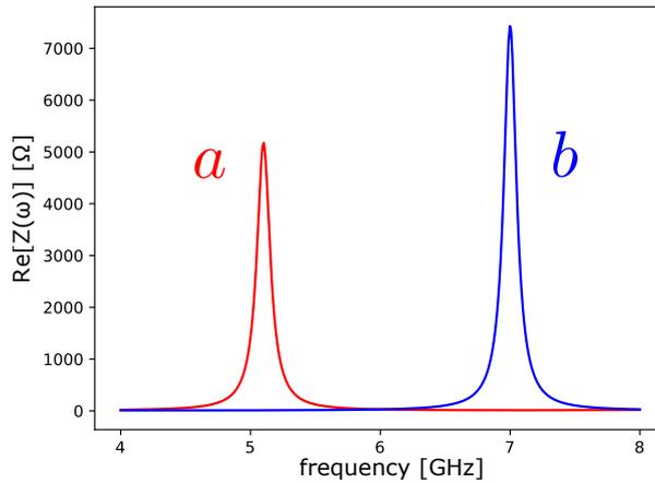
Figure 4.15: Impedance seen on each side of the junction, computed with the transmission line formula for impedance transforms [118]. The two modes at 5.1 GHz and 7.0 GHz have similar FWHM  $\simeq 120$  MHz.
