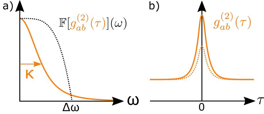
Figure 4.39: a) The Fourier transform of  $g_{ab}^{(2)}(\tau)$  is a Lorentzian function of width  $\kappa$  at low driving  $\beta \ll 1$ . The bandpass filtering used in the experiment amounts to low-pass filtering  $\mathbb{F}[g_{ab}^{(2)}(\tau)](\omega)$ . The shape of the low-pass filter (dashed) depends on the detail of the bandpass filters. b) The measured correlator of filtered signals (dashed curve) shows less correlations than for the unfiltered fields (full curve).
