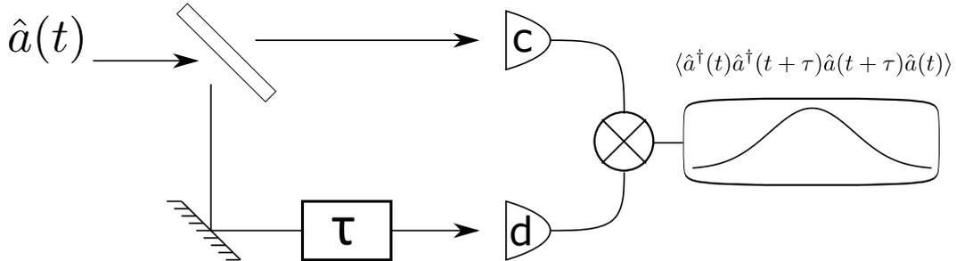
Figure 3.16: Hanbury Brown-Twiss (HBT) interferometer. The field  $\hat{a}(t)$  is split onto two different paths. The intensity of the two beams is measured by two photo-counters. The product of the two photo-currents is  $\propto g^{(2)}(\tau)$ .
