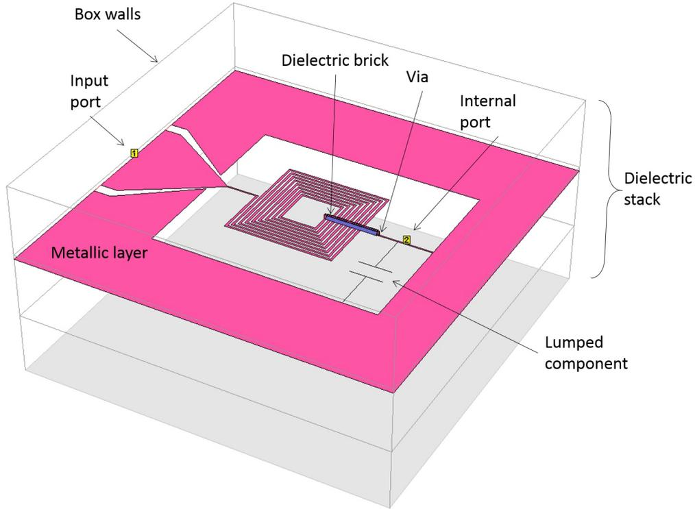
Figure 3.8: Model used in a Sonnet simulation, implementing the circuit of figure 3.7. The Josephson junction (not shown) is placed at port 2 between the ground and the coil, and is shunted by  $C_J$ , which is modelled as a lumped capacitor component of 2 fF. The coil (square in this iteration of the design) is connected to the detection chain at the input port 1, and to the junction through a bridge supported by a micron-thick dielectric bridge (taken from [35]).
