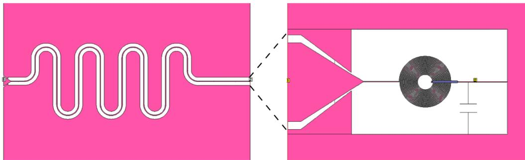
Figure 3.9: Final design for the strong-coupling resonator. A  $240 \mu\text{m}$  wide coil is made with 23 turns of a  $1 \mu\text{m}$  wire with  $2 \mu\text{m}$  spacings between the turns. One port of the coil is connected to a  $70 \Omega \lambda/4$  resonator, that raises the input impedance seen by the coil up to  $100 \Omega$  at 5 GHz. The inner pad is connected via a supported bridge to a grounded Josephson junction (taken from [35]).
