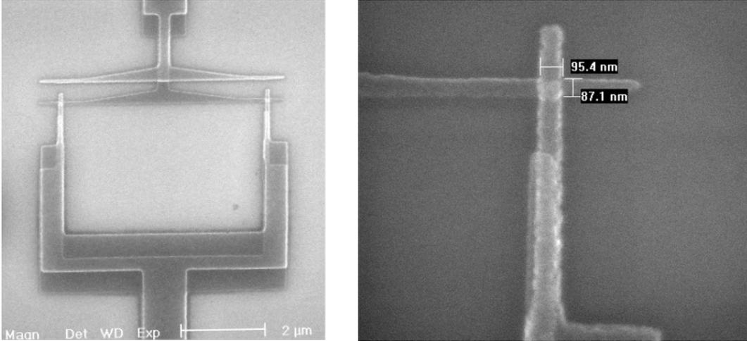
Figure 3.12: Scanning Electron Microscopy image of the nanofabricated SQUID. The two  $\sim 100 \times 100 \text{ nm}^2$  junctions are expected to add around 2 fF of geometric capacitance to the mode (taken from [35]).
