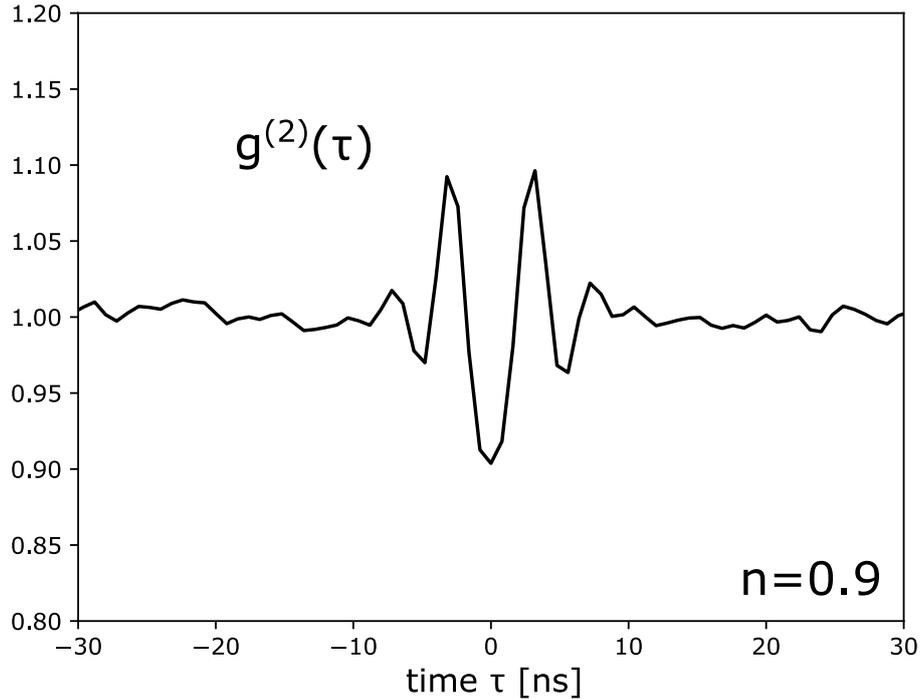
Figure 3.62: Second order coherence function at the highest emission rate, where  $\bar{n} = 0.9$ . We attribute the ripples to Rabi oscillations between the cavity field and the tunneling Cooper pairs.
