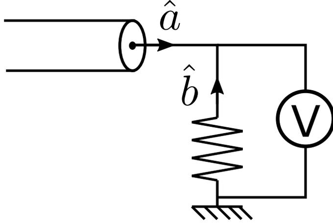
Figure 3.23: Gedanken experiment: measuring directly the fast voltage drop resulting from photons impinging on a load resistor. Even if the voltmeter is fast enough it will not detect  $\hat{a}$ , but a combination of  $\hat{a}$  and an added noise term  $\hat{b}^\dagger$ .
