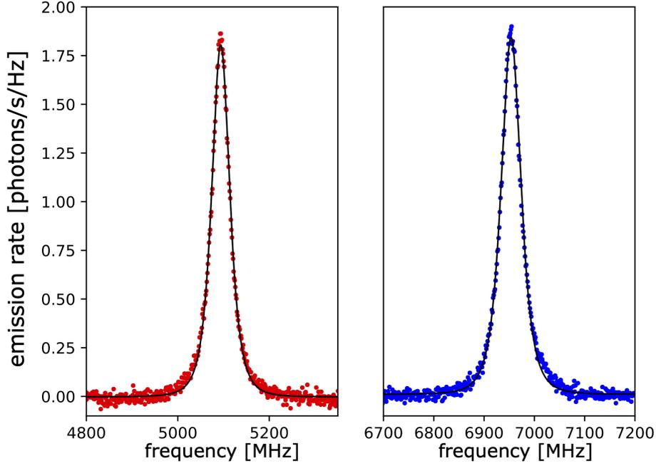
Figure 4.27: Emission spectra at a voltage bias  $2eV = h \times 12.05$  GHz. The spectra are fitted by a Lorentzian function squared, reproducing the  $Re[Z(\omega)] \times Re[Z(\omega_J - \omega)]$  shape.
