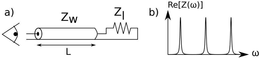
Figure 2.11: a) The impedance  $Z_l$  seen through some length  $L$  of transmission line  $Z_w$  shows resonances. b) If  $Z_w > Z_l$ , these resonances happens at odd multiples of the fundamental resonant frequency. The impedance on top of the resonance is  $Z_w^2/Z_l$ , and the quality factor is  $Q = \pi Z_w/4Z_l$ .
