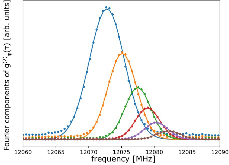
Figure 4.40: Gaussian fits of the Fourier transforms of the phase correlators, measured at occupation numbers ranging from  $\bar{n} = 0.33$  (blue points and curve) down to  $\bar{n} = 0.033$  (brown points and curve).
