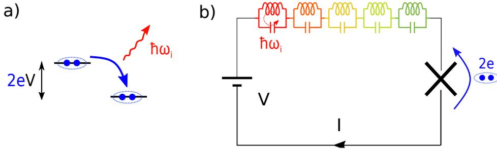
Figure 1.4: a) Schematic picture of a Cooper pair inelastically tunneling through a dc-biased junction while emitting a photon of energy  $\hbar\omega_i = 2eV$ . b) The energy to create a photon in a mode of the environment (depicted here as a collection of  $LC$  oscillators) is extracted from the voltage source  $V$ .
