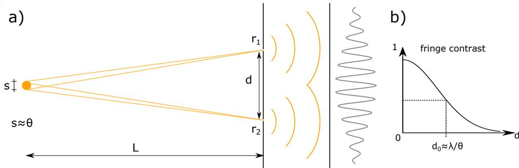
Figure 3.14: a) Schematics of a Michelson-like stellar interferometer. A star with angular diameter  $\theta$  illuminates a Young slits setup. The spacing of the fringes is linked to the wavelength of the light, while their visibility (b) depends on  $\theta$  and the spacing of the slits  $d$ .
