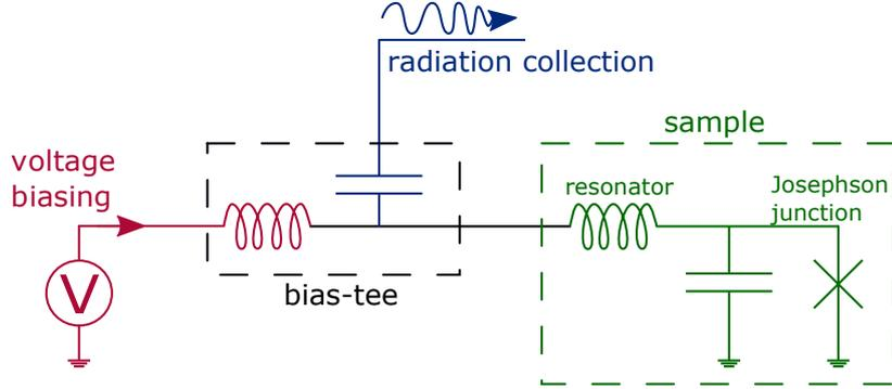
Figure 3.13: Principle of the experiment: the Josephson junction is dc-biased through the high-impedance resonator. A bias-tee at the output of the sample routes the microwave signals leaking out of the resonator towards the detection chain, while allowing the application of a precise voltage bias  $V$  (taken from [35]).
