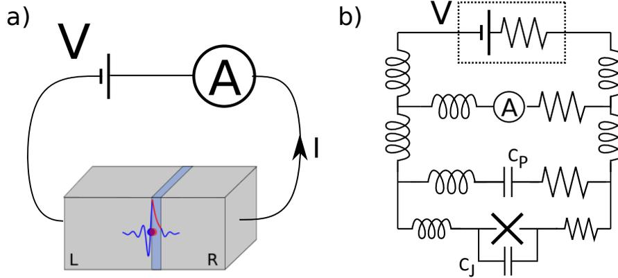
Figure 2.4: a) Ideal tunnel junction  $I(V)$  measurement setup. b) Model of a more realistic version including the internal voltage source resistance, the inductance of the dissipative leads going to the Josephson junction (represented here and after by a  $\times$  symbol), the parasitic shunt capacitances of the bonding pads  $C_P$  and the geometric capacitance of the junction  $C_J$ .
