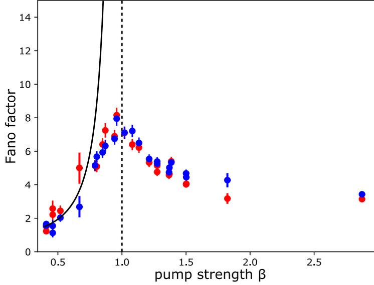
Figure 4.33: Fano factors of the  $a$  (red dots) and  $b$  (blue dots) photons as a function of the reduced pump strength. As  $\beta$  is increased, the Fano factors increase strongly from about 1.5 at low driving to 8 near the parametric transition threshold. Above the threshold, they decrease slowly. The parametric model prediction (black line) diverges at  $\beta = 1$ .
