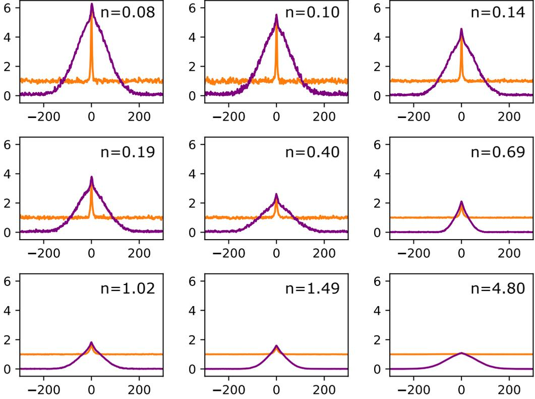
Figure 4.43: Measurement of the entanglement witness correlators  $g_{ab}^{(2)}(\tau)$  (orange curves) and  $|g_{\phi}^{(2)}(\tau)|$  (purple curves) as a function of time  $\tau$  in nanoseconds, for  $\bar{n}$  ranging from 0.08 up to 4.8.
