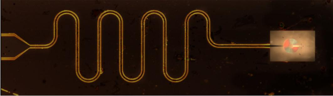
Figure 3.10: Optical image of the whole 3 mm×10 mm chip, showing the impedance adaptation resonator (meanders in the middle) and the bonding pad on the left (taken from [35]).
