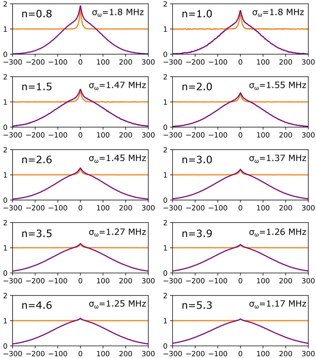
Figure 4.50: Entanglement correlators measured in the cooling regime. As the pump strength  $\beta$  is increased, the  $\tau = 0$  value of correlators decreases down to 1. At the same time the dephasing rate  $\sigma_\omega$  is reduced, due to cooling of the low frequency modes by the junction.
