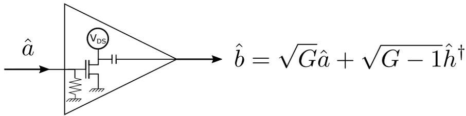
Figure 3.20: Quantum model of a linear amplifier, as described by [81]. The amplified signals are carried by an output mode  $\hat{b}$ , which also includes noise contribution from a mode  $\hat{h}^\dagger$ . The details and physical origin of  $\hat{h}^\dagger$  depend on the specific implementation of the amplifier (here thermal noise from an internal resistance).
