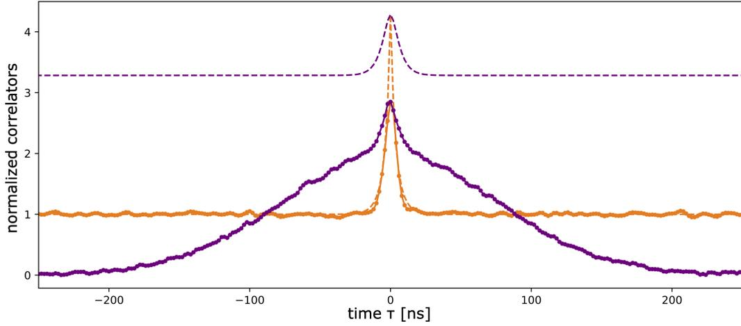
Figure 4.38: Correlation functions  $g_{ab}^{(2)}(\tau)$  (orange points) and  $|g_\phi^{(2)}(\tau)|$  (purple points) measured at an occupation number  $\bar{n} = 0.22$ , with theoretical predictions of the parametric model (dashed curves).
