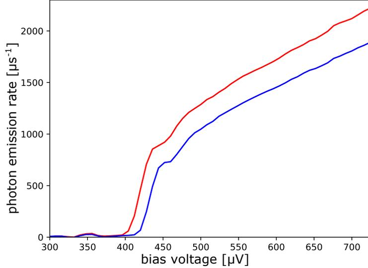
Figure 4.22: Total emission rate in the  $a$  mode (red curve) and the  $b$  mode (blue curve) as a function of the bias voltage. At bias voltage  $V = (2\Delta + \hbar\omega_0)/e$  larger than the gap voltage, quasiparticles can tunnel through the junction, generating shot-noise with a spectral density  $S_{II}(\omega) \neq 0$  for  $\omega \leq \omega_0$ . The emission power at  $\omega_a$  is thus shifted by  $(\omega_b - \omega_a)/e$  with respect to the emission power at  $\omega_b$ .
