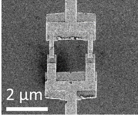
Figure 4.17: Electronic micrography image of the SQUID connected between the two resonators.
