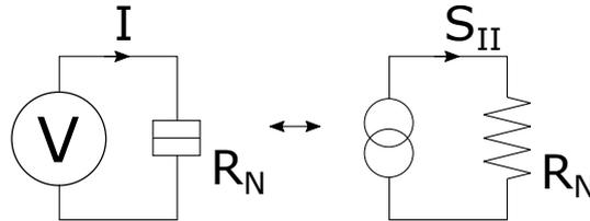
Figure B.2: A dc-biased tunnel junction give rise to a tunnel current, which includes an average value  $\bar{I} = V/R_N$  as well as a noise spectral density  $S_{II}(\omega)$ .
