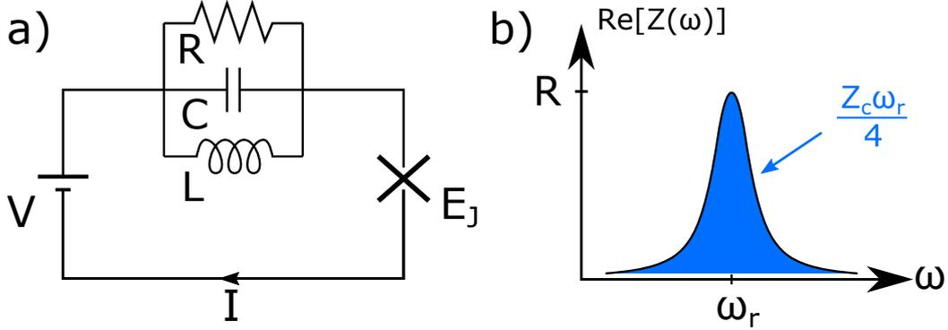
Figure 3.1: a) Model circuit: a Josephson junction with energy  $E_J$  is dc-biased by a voltage source  $V$  through a  $RLC$  resonator with frequency  $\omega_r = 1/\sqrt{LC}$ , characteristic impedance  $Z_c = \sqrt{L/C}$  and quality factor  $Q = R/Z_c$ . b)  $Re[Z(\omega)]$  of the environment of the junction.  $Z_c$  is proportional to its integral.
