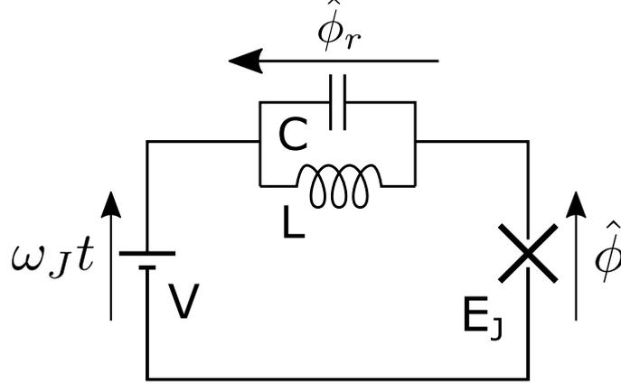
Figure 3.2: A dc-biased Josephson junction coupled to a single  $LC$  mode, with notations for the phase operators across each element of the circuit.
