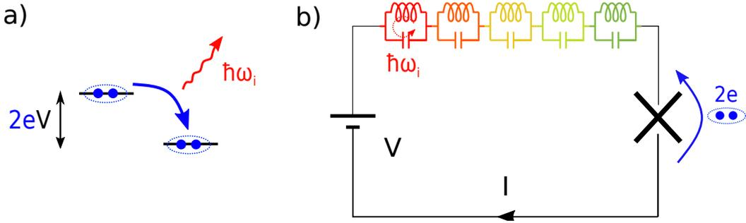
Figure 2.9: a) If  $2eV = \hbar\omega_i$ , a Cooper pair can tunnel inelastically and create one photon at frequency  $\omega_i$ . b) There is then a dc-current flowing in the circuit, associated to the dissipation of ac-power in the environment.
