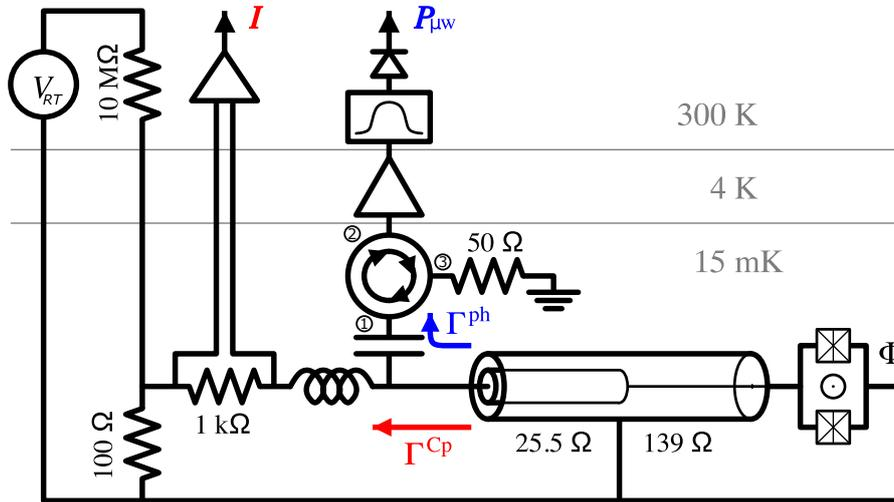
Figure 2.14: Generic setup used in the 2011 experiment. A bias tee allows to measure the dc-current of Cooper pairs  $\Gamma_{Cp}$  as well as collecting the microwave power  $\Gamma_{ph}$  emitted into an amplification chain.
