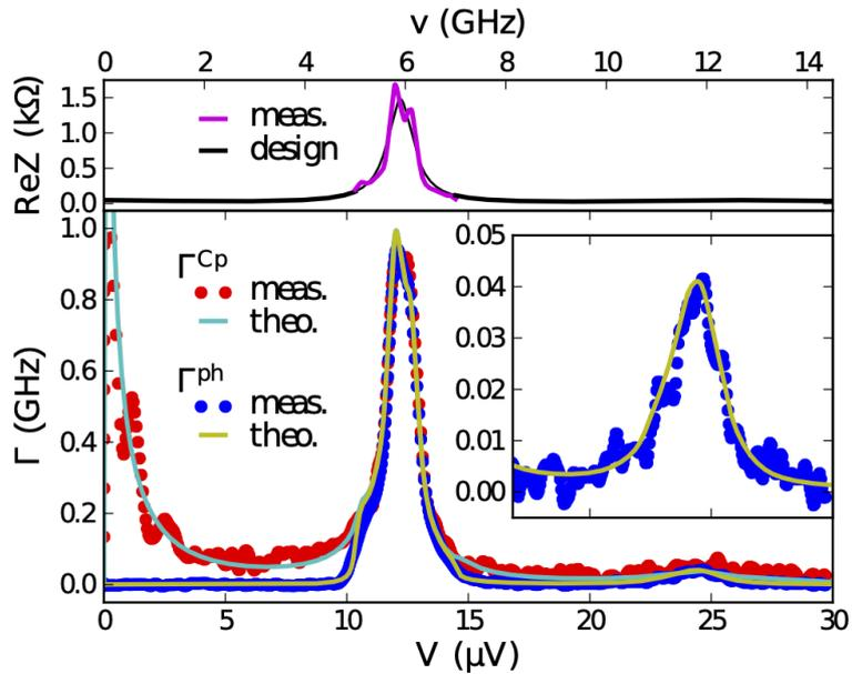
Figure 1.6: Results of the experiment described in [33], where both the Cooper pair tunneling rate  $\Gamma_{Cp}$  and the photon emission rate  $\Gamma_{ph}$  in a mode at  $\omega_r/2\pi = 6$  GHz were measured. On the 1-photon resonance  $2eV = \hbar\omega_r$ ,  $\Gamma_{Cp}$  and  $\Gamma_{ph}$  coincide. On the 2-photon resonance  $2eV = 2\hbar\omega_r$ , the emission power at  $\omega_r$  is detected, indicating 2-photon processes (inset).
