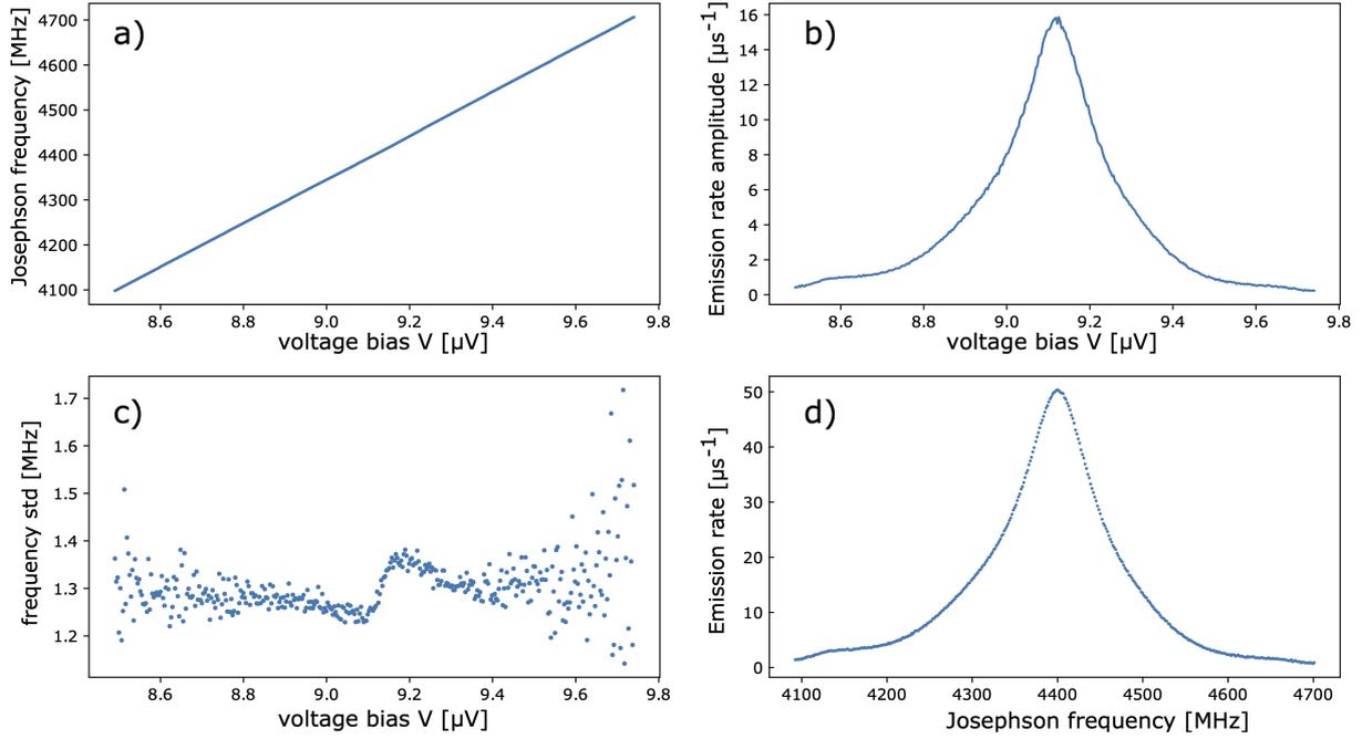
Figure 3.40: Results of the gaussian fits of spectra from figure 3.34. As a function of the bias voltage  $V$ , panel a), b) and c) show the fitted Josephson frequencies, peak amplitudes and standard deviations. Panel d) combines results of the fits to display the emission rate (proportional to  $Re[Z(2eV/h)]$ ) as a function of the Josephson frequency.
