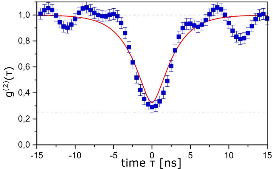
Figure 3.19: Results from the 2016 experiment. Values of  $g^{(2)}(\tau)$  measured *via* power fluctuation correlations (blue squares) on top of the theoretical prediction of [34]:  $g^{(2)}(\tau) = (1 - re^{-\kappa\tau}/2)^2$ , with a fitted  $r = 1$  and  $\kappa = 1 \text{ ns}^{-1}$ . The error bars indicate half the statistical standard deviation,  $\sigma/2$  (taken from [35]).
