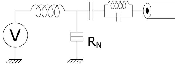
Figure B.1: Model circuit of the experiments in the shot-noise regime. Biased far above the gap voltage, the Josephson junction behaves as a normal junction with tunnel resistance  $R_N$  (box symbol). A bias-tee defines low-frequency and rf branches of the rest of the circuit, with a dc resistance  $Re[Z(0)] = 0$ .
