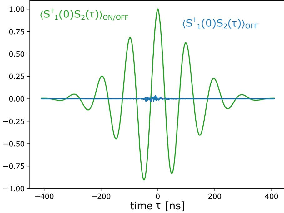
Figure 3.55: Real part of the normalized first order correlators. The *ON/OFF* correlator yields the  $g^{(1)}(\tau)$  function of the signals (in green). The *OFF* correlator shows the parasitic coupling between the two channels (in blue).
