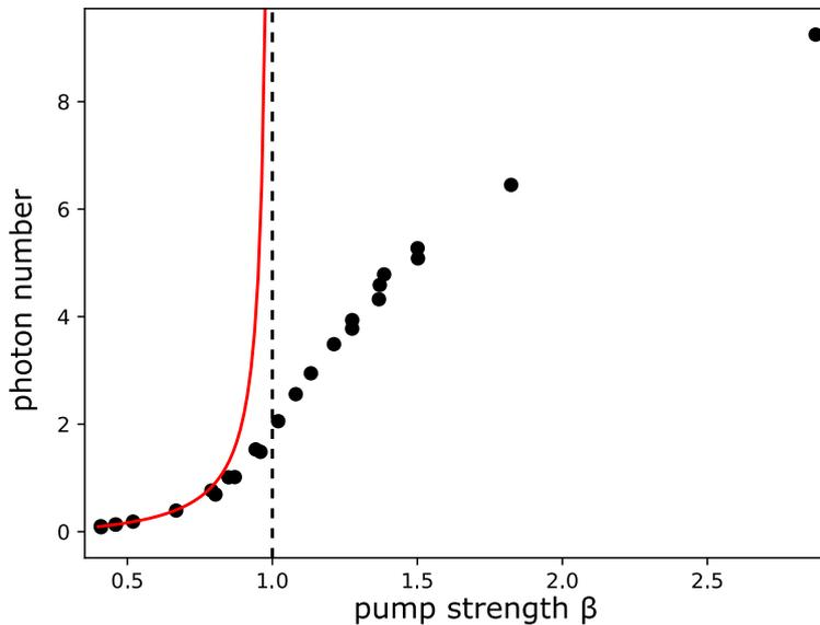
Figure 4.30: Occupation number of the cavities  $\bar{n}$  as a function of the pump strength  $\beta$ . The measured values (black dots) agree well with the parametric amplifier model (red line) at low  $\beta$ . Close to the parametric transition  $\beta = 1$ , the simple model predicts a divergence of  $\bar{n}$ . In the real system.
