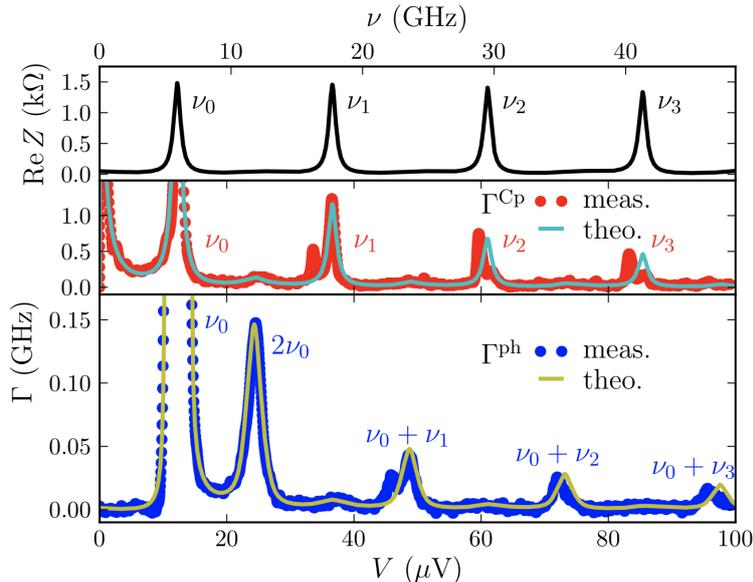
Figure 2.16: Results of the experiment at higher bias. The upper graph shows  $Re[Z(\nu)]$  as it was designed, with harmonics of the  $\lambda/4$  resonance at frequencies  $\nu_k = (2k+1)\nu_0$ . To these modes correspond 1-photon peaks in  $\Gamma_{Cp}$ , at bias voltages  $V = h\nu_k/2e$ . We see 2-photon peaks in  $\Gamma_{ph}$ , at voltages  $V = h(\nu_k + \nu_0)/2e$ .
