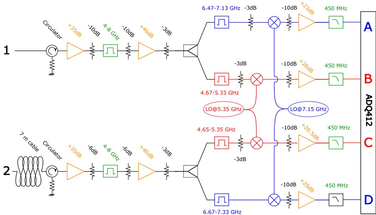
Figure 4.19: Room-temperature setup. After amplification, filtering and down-conversion,  $a$  and  $b$  signals carried by the two channels (1) and (2) are separated by bandpass filtering and detected separately on four acquisition channels. The attenuation and length of each channel is adjusted to yield balanced signal powers and propagation times.
