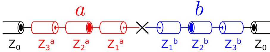
Figure 4.14: Microwave electrical model of the sample. The small Josephson junction acts as an open circuit. The segments of CPW on the left (right) side have a length such that their first  $\lambda/4$  resonance occurs at  $\omega_a$  ( $\omega_b$ ).
