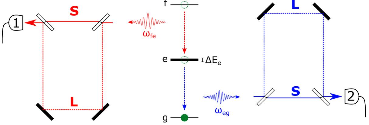
Figure 4.10: Original Franson experiment. An atom (green dot) undergoes a relaxation cascade, emitting successively two photons (red and blue wavepackets). Each photon is routed towards an unbalanced Mach-Zehnder interferometer. The imbalance of the short (S) and long (L) paths is larger than the one-photon coherence length. Nevertheless, coincidences of the detection rates at photo-counters (1) and (2) reveal non-classical two-photon coherence.
