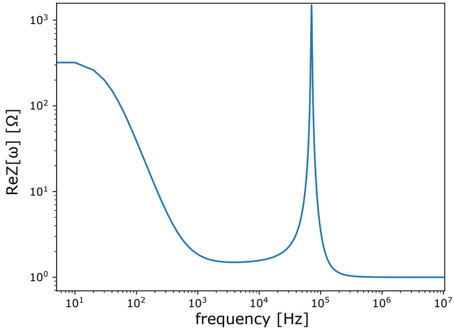
Figure 3.36: Model for the low-frequency impedance seen of the environment.  $R_3$  gives the dc resistance of the bias line. It gets shunted above 70 Hz by the  $6.6 \mu\text{F}$  capacitance put in parallel. At 71 kHz lies the self resonance of the bias-tee, with a  $53 \Omega$  impedance and a quality factor of the order of 30. At higher frequencies the cavity filter shunts the impedance to about  $1 \Omega$ .
