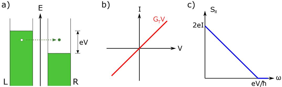
Figure 2.2: a) Schematic energy bands in a metallic tunnel junction at zero temperature. A bias voltage  $V$  shifts the two Fermi levels by  $eV$ . Irreversible elastic tunneling occurs when an electron jumps from an occupied state to an empty one. b)  $I(V)$  characteristic of a metallic tunnel junction. c) Current shot-noise  $S_{II}(\omega)$  of a tunnel junction at zero temperature.
