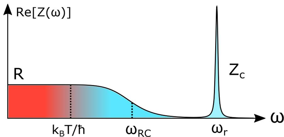
Figure 2.18: Environment of a dc-biased Josephson junction: near zero frequency is a continuum of states with high thermal population, while at  $\omega_r$  is a mode of characteristic impedance  $Z_c$  in the vacuum state. Color-coded is the thermal occupation of modes, which drops to zero above  $k_B T / \hbar$ .
