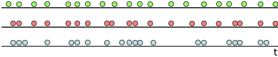
Figure 3.5: Schematic picture of the photons in a beam of light displaying (from top to bottom) anti-bunching, classical and bunchings statistics.
