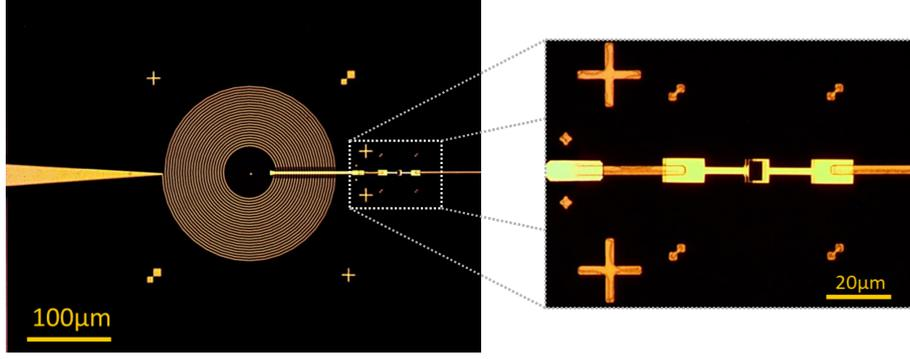
Figure 1.9: Micrograph of the sample fabricated by Chloé Rolland during her PhD. The microfabricated coil (left part) implements a resonator in the strong-coupling regime with a SQUID-like tunable JJ (inset), with  $r \simeq 1$ .
