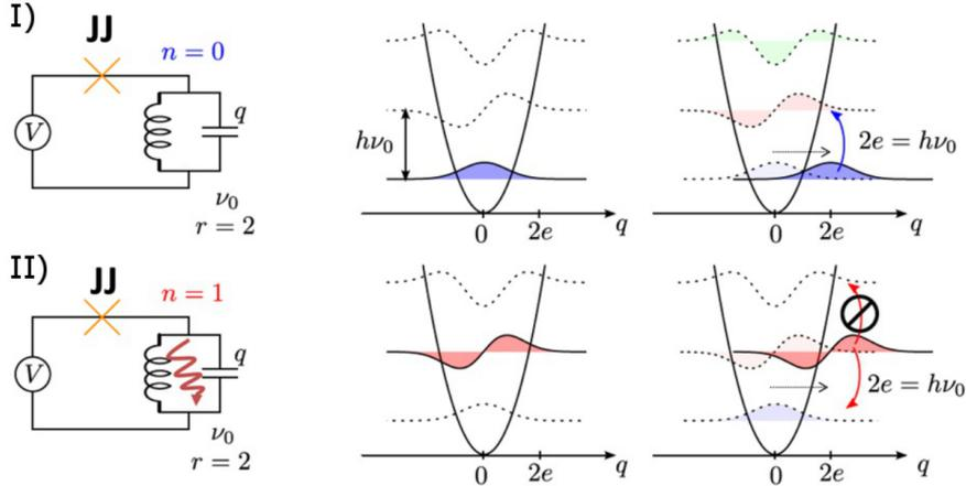
Figure 1.8: Photon blockade mechanism in a mode strongly coupled to a JJ with  $r = 2$ . After a single Cooper pair has tunneled, the mode ends up in its first excited state, with a wavefunction displaced in charge space by  $q = 2e$ . This displaced wavefunction does not overlap with the next excited state, so that the creation of a second photon is forbidden.
