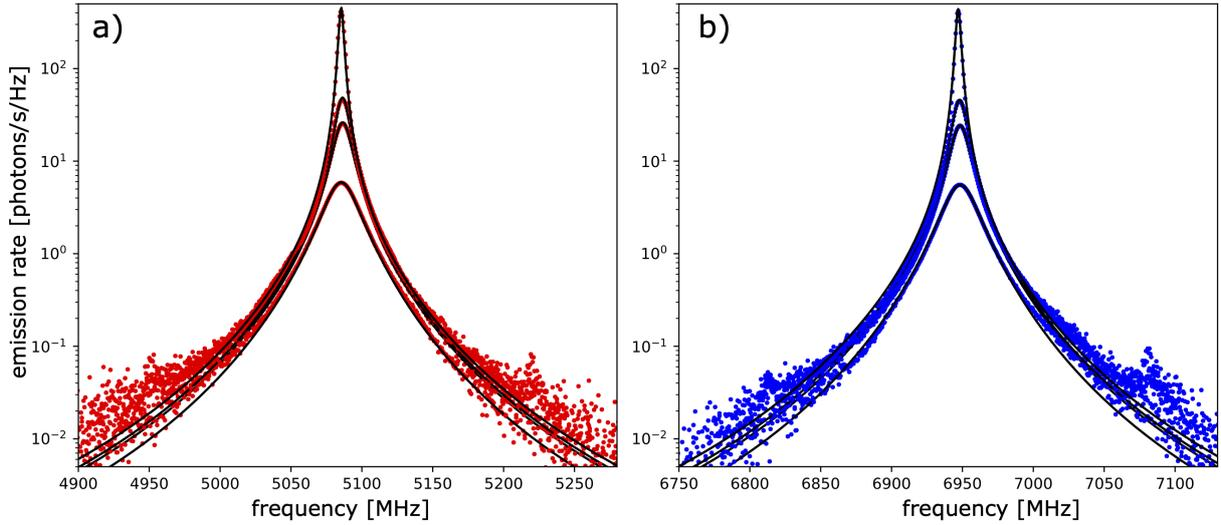
Figure 4.28: Emission spectra at a voltage bias  $2eV = h \times 12.035$  GHz and increasing pump strength  $\beta$ . The independent fits in panels (a) and (b) yield the same value of the detuning  $\Delta \simeq -10$  MHz and of the emission rates, corresponding to  $\bar{n} = 0.4, 1.0, 1.5$  and  $5.0$  photons respectively ( $\pm 5\%$ ).
