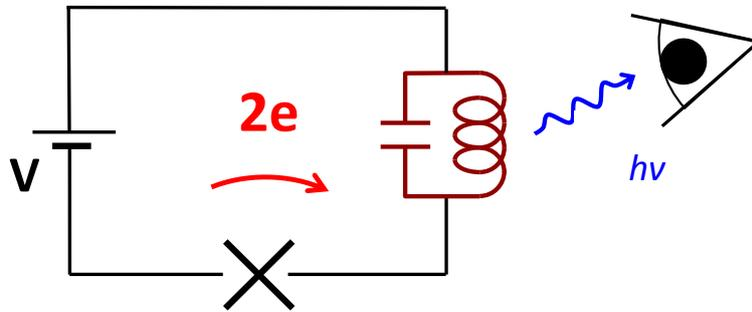
The coupling between a dc-biased Josephson junction and a single mode with a high characteristic impedance  $Z_c$  yields a situation with no direct equivalent in atomic QED, as the fine-structure constant  $r = \pi Z_c / R_Q$  can be made of the order of 1. The light-matter interaction is then considerably modified compared to the weakly-coupled regime: if a charge emits a photon, the back-action of the photon on the charge is large enough to modify its dynamics.
