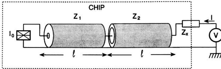
Figure 2.10: Circuit used by Holst *et al.* for the 1994 experiment. An ultrasmall Josephson junction (box symbol  $\boxtimes$ ) is connected to a voltage source through two segments of transmission line built on-chip.
