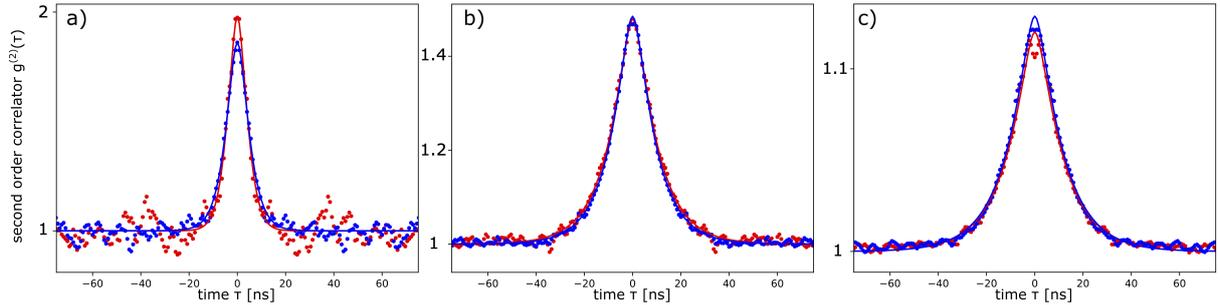
Figure 4.31: Second order coherence functions of the  $a$  (red) and  $b$  (blue) photons, measured at occupation numbers of  $\bar{n} = 0.13$  (panel a),  $1.0$  (panel b) and  $3.0$  (panel c) photons, with phenomenological fits.
